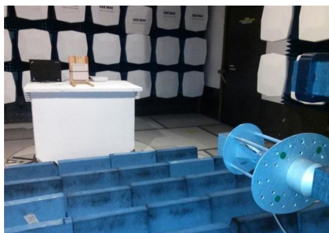
Radiated Emissions (>18 GHz) – Front View
