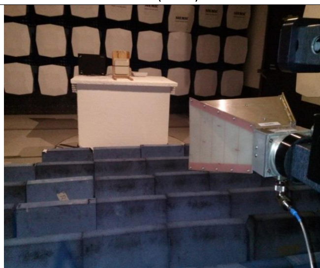
Radiated Emissions (>1GHz) – Front View
