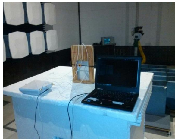
Radiated Emissions (>18 GHz) – Rear View
