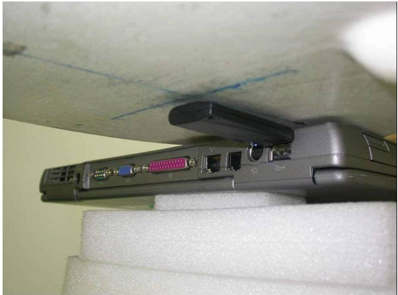
**The Bottom of the EUT to the flat phantom distance 2 mm**
