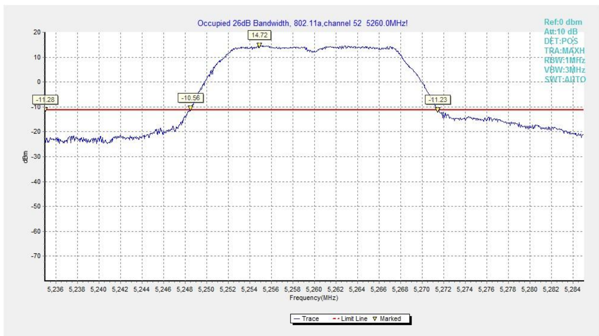
Fig. 4 Occupied 26dB Bandwidth (802.11a, 5260MHz)
