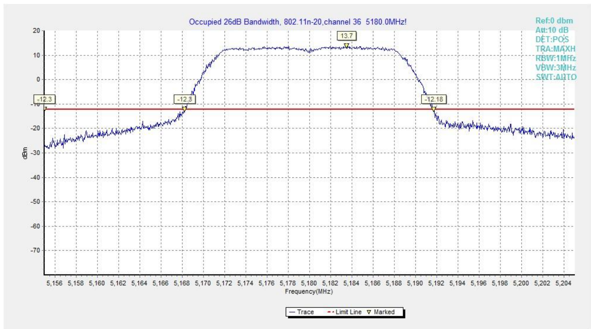
Fig. 10 Occupied 26dB Bandwidth (802.11n-HT20, 5180MHz)
