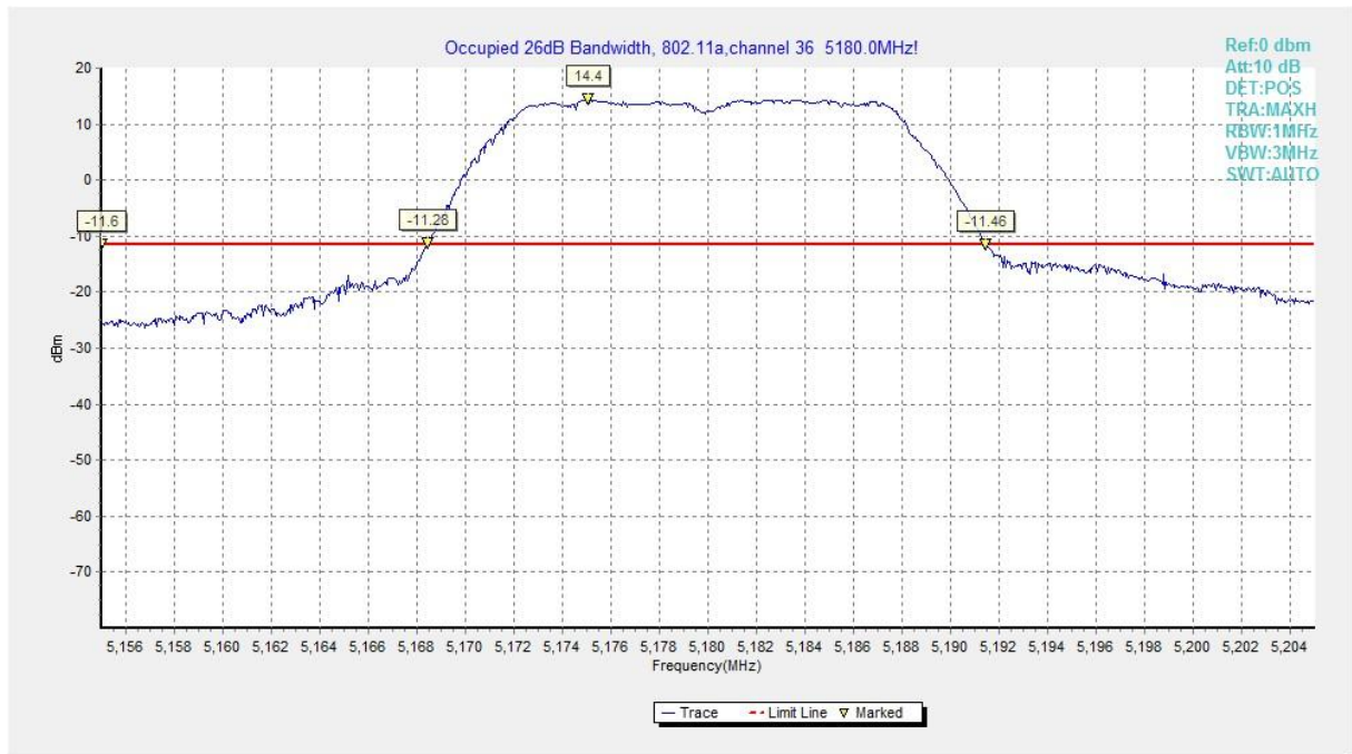
Fig. 1 Occupied 26dB Bandwidth (802.11a, 5180MHz)
