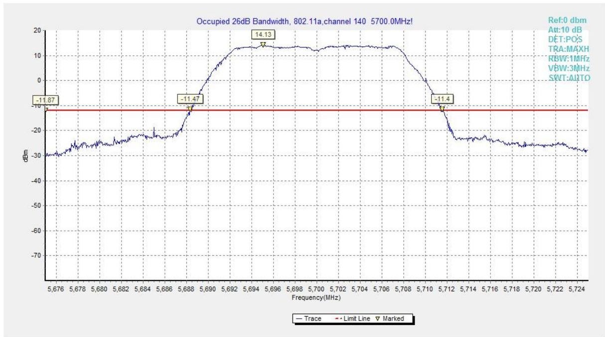
Fig. 9 Occupied 26dB Bandwidth (802.11a, 5700MHz)
