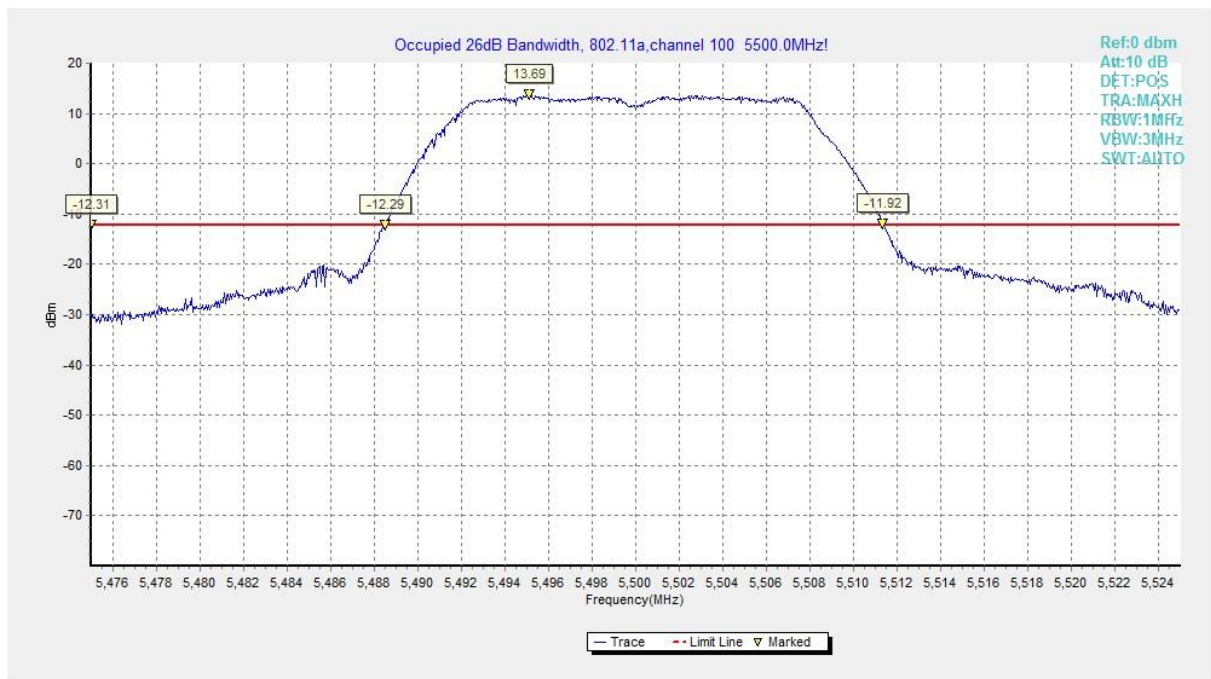
Fig. 7 Occupied 26dB Bandwidth (802.11a, 5500MHz)
