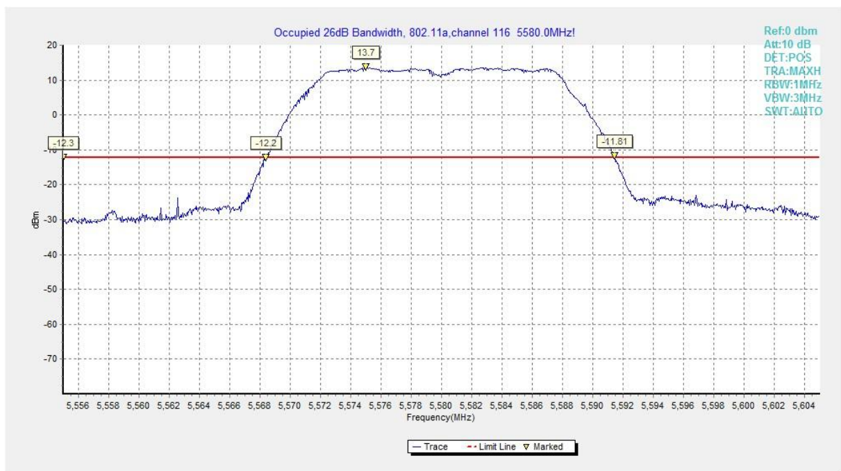
Fig. 8 Occupied 26dB Bandwidth (802.11a, 5580MHz)
