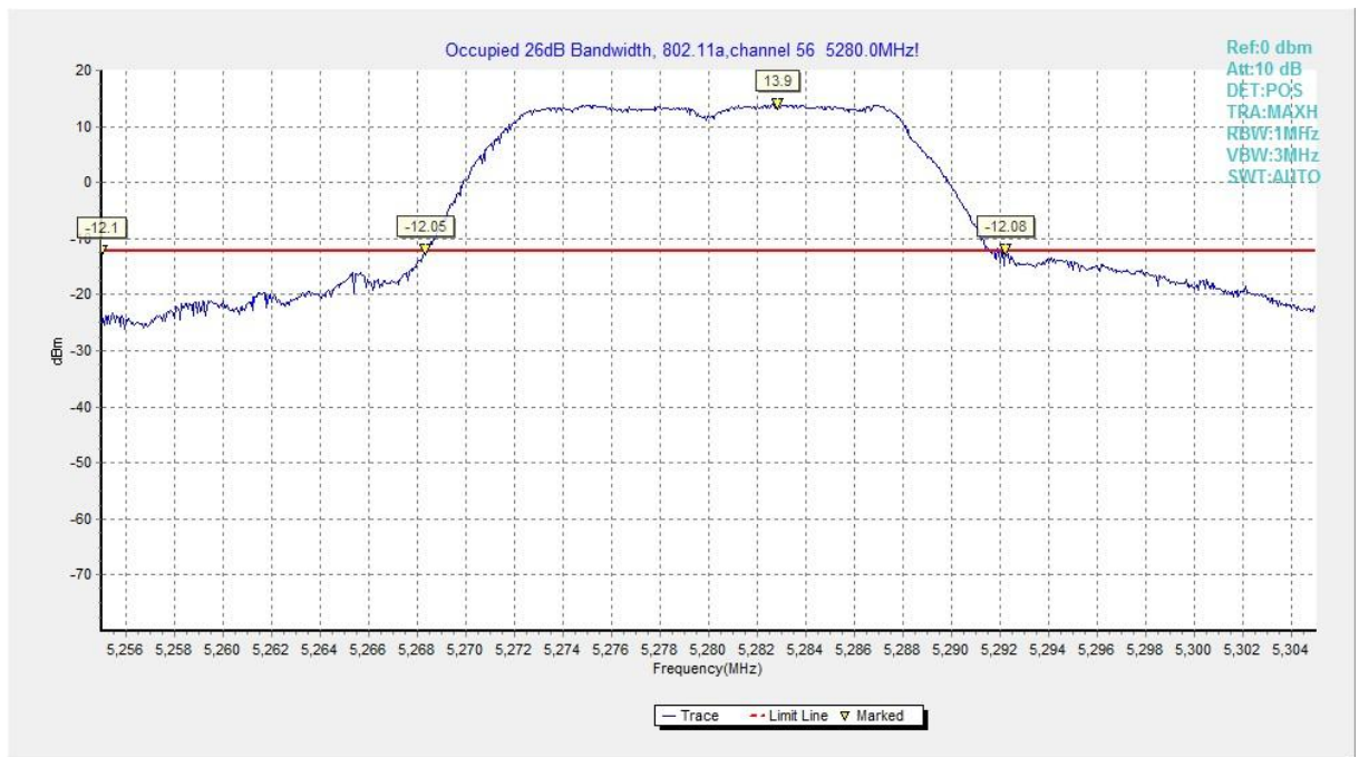
Fig. 5 Occupied 26dB Bandwidth (802.11a, 5280MHz)
