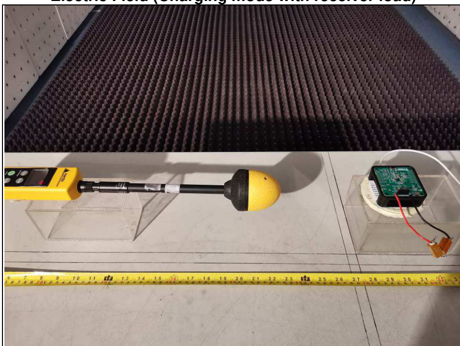
Electric Field (Charging mode with receiver load)
