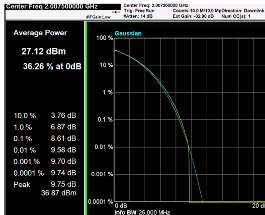
Channel: MIDDLE, Modulation: 256QAM, BW=15MHz, CCDF
