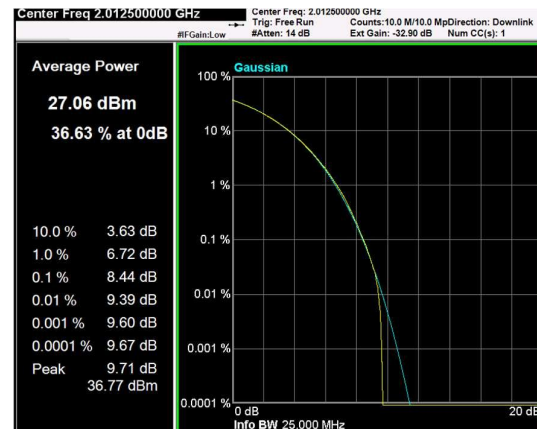
Channel: TOP, Modulation: 16QAM, BW=15MHz, CCDF
