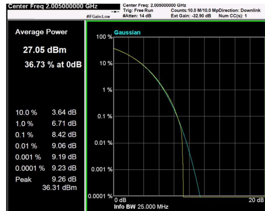
Channel: BOTTOM, Modulation: 64QAM, BW=20MHz, CCDF
