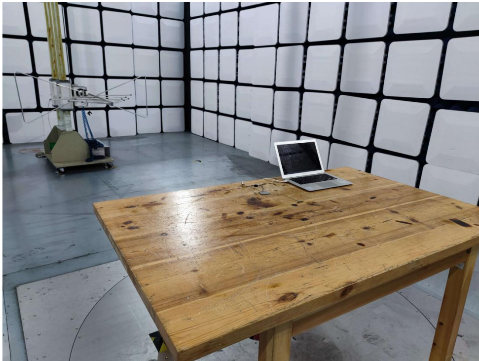
Photo of Radiation Emission Test
