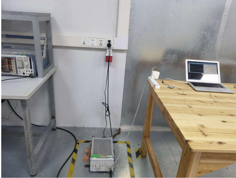
Photo of Power Line Conducted Emission Test
