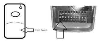
3. Using a paper clip or pen match the code to your receiver which was determined in step 1. The switch has an on and off position which is selected by gently pressing up or down.
