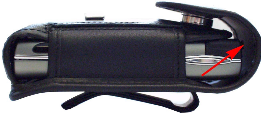
Picture 7. LJPNSB-6NY placed in Carrying Case from CBP-2 and the position of the antenna
