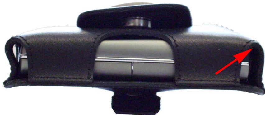
Picture 5. LJPNSB-6NY placed in CSH-3 and the position of the antenna
