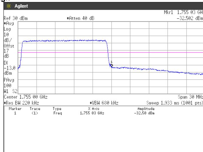
**16QAM, BW 20MHz, RB1-0****Channel: Low**
