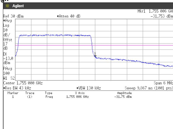
**16QAM, BW 5MHz, RB1-0****Channel: Low**
