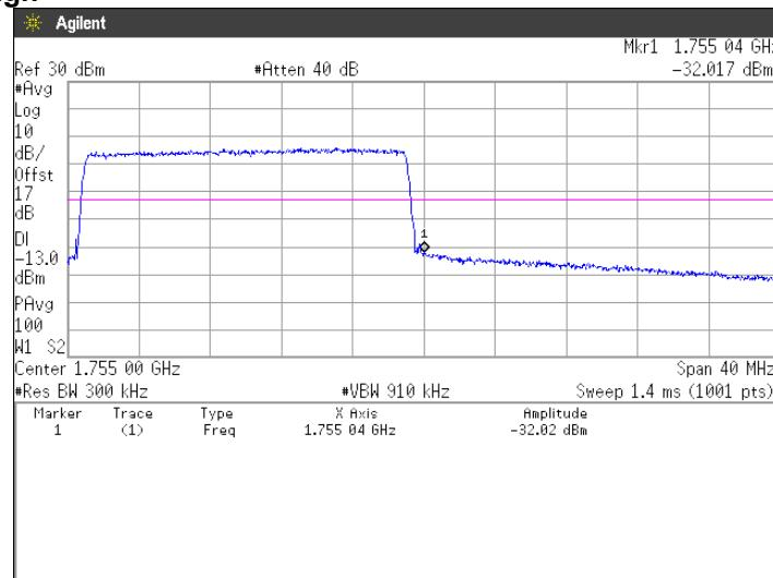
**16QAM, BW 1.4MHz, RB1-0****Channel: Low**
