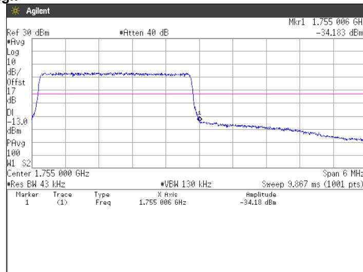
**64QAM, BW 5MHz, RB1-0****Channel: Low**
