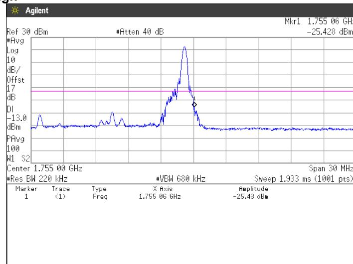
**QPSK, BW 15MHz, RB75-0****Channel: Low**
