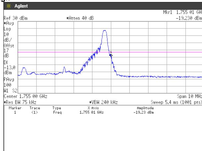
**64QAM, BW 5MHz, RB25-0****Channel: Low**
