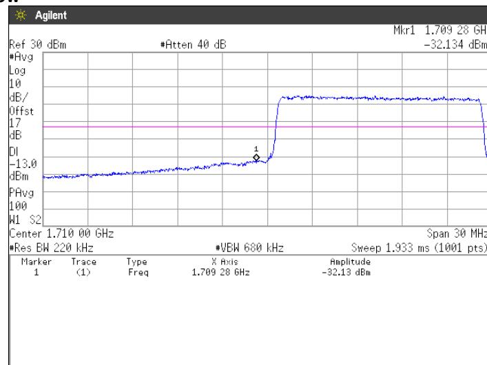
**16QAM, BW 15MHz, RB75-0****Channel: High**
