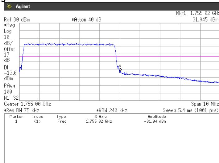
**16QAM, BW 10MHz, RB1-0****Channel: Low**
