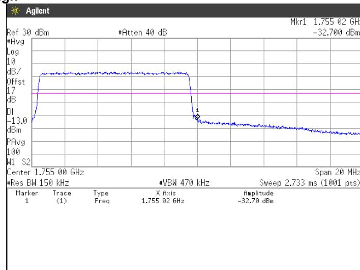
**64QAM, BW 15MHz, RB1-0****Channel: Low**
