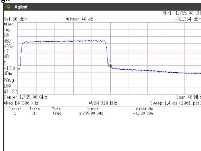
**64QAM, BW 1.4MHz, RB1-0****Channel: Low**
