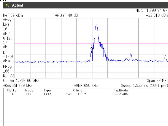
**64QAM, BW 15MHz, RB1-74****Channel: High**
