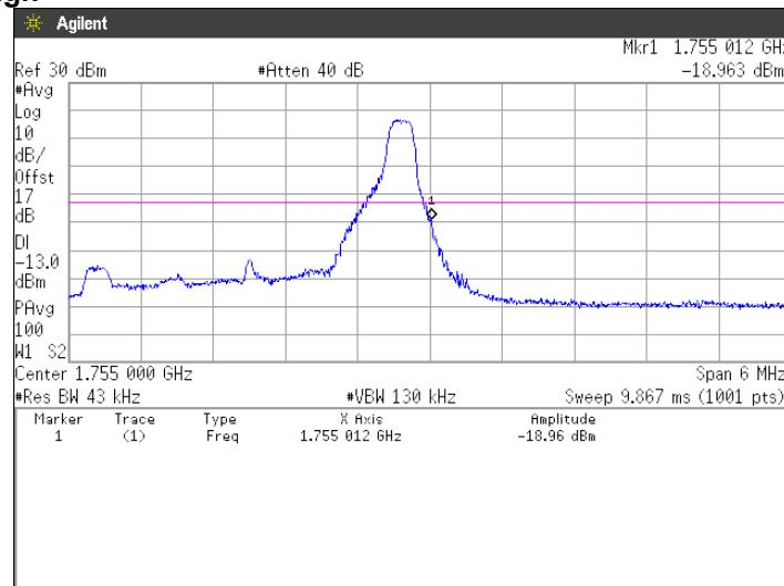
**16QAM, BW 3MHz, RB15-0****Channel: Low**
