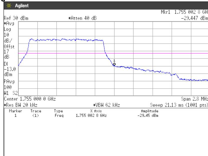
**QPSK, BW 3MHz, RB1-0****Channel: Low**
