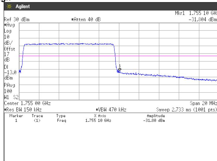
**QPSK, BW 15MHz, RB1-0****Channel: Low**
