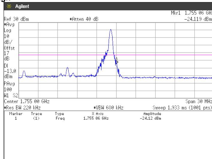
**64QAM, BW 15MHz, RB75-0****Channel: Low**
