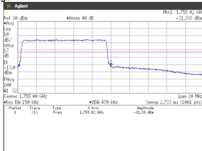
**16QAM, BW 15MHz, RB1-0****Channel: Low**
