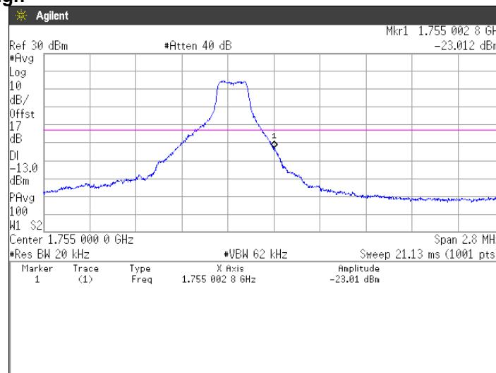
**QPSK, BW 1.4MHz, RB6-0****Channel: Low**
