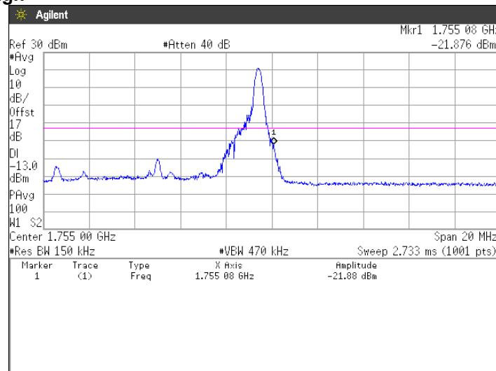
**16QAM, BW 10MHz, RB50-0****Channel: Low**
