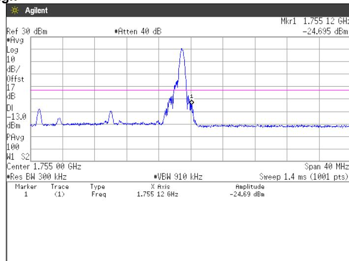
**64QAM, BW 20MHz, RB100-0****Channel: Low**
