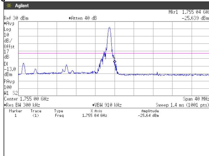
**QPSK, BW 20MHz, RB100-0****Channel: Low**
