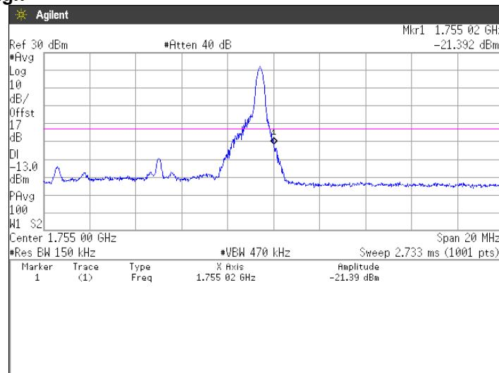
**QPSK, BW 10MHz, RB50-0****Channel: Low**
