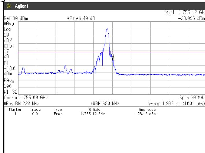
**16QAM, BW 15MHz, RB75-0****Channel: Low**
