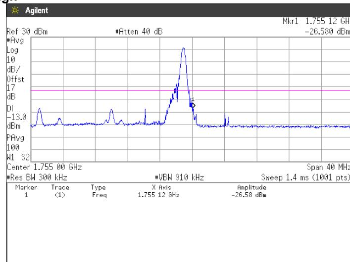
**16QAM, BW 20MHz, RB100-0****Channel: Low**
