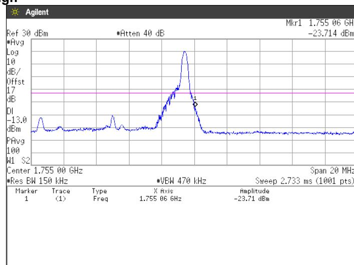
**64QAM, BW 10MHz, RB50-0****Channel: Low**
