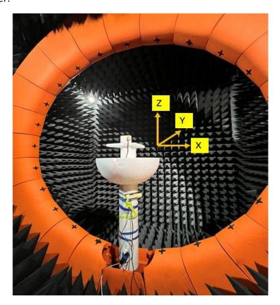
2. Laser pointer centered on BLE antenna
