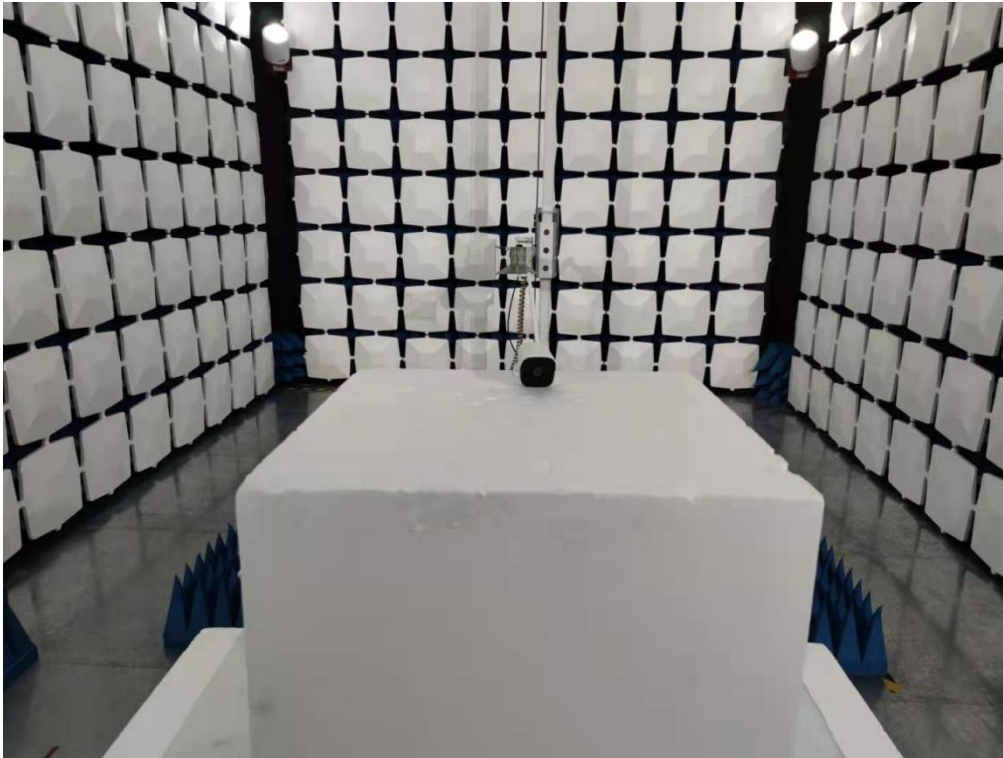
Above 1GHz for radiated emission test setup
