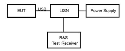
Note: Power Supply is AC Power source and it is used to change the voltage 120V/60Hz.
