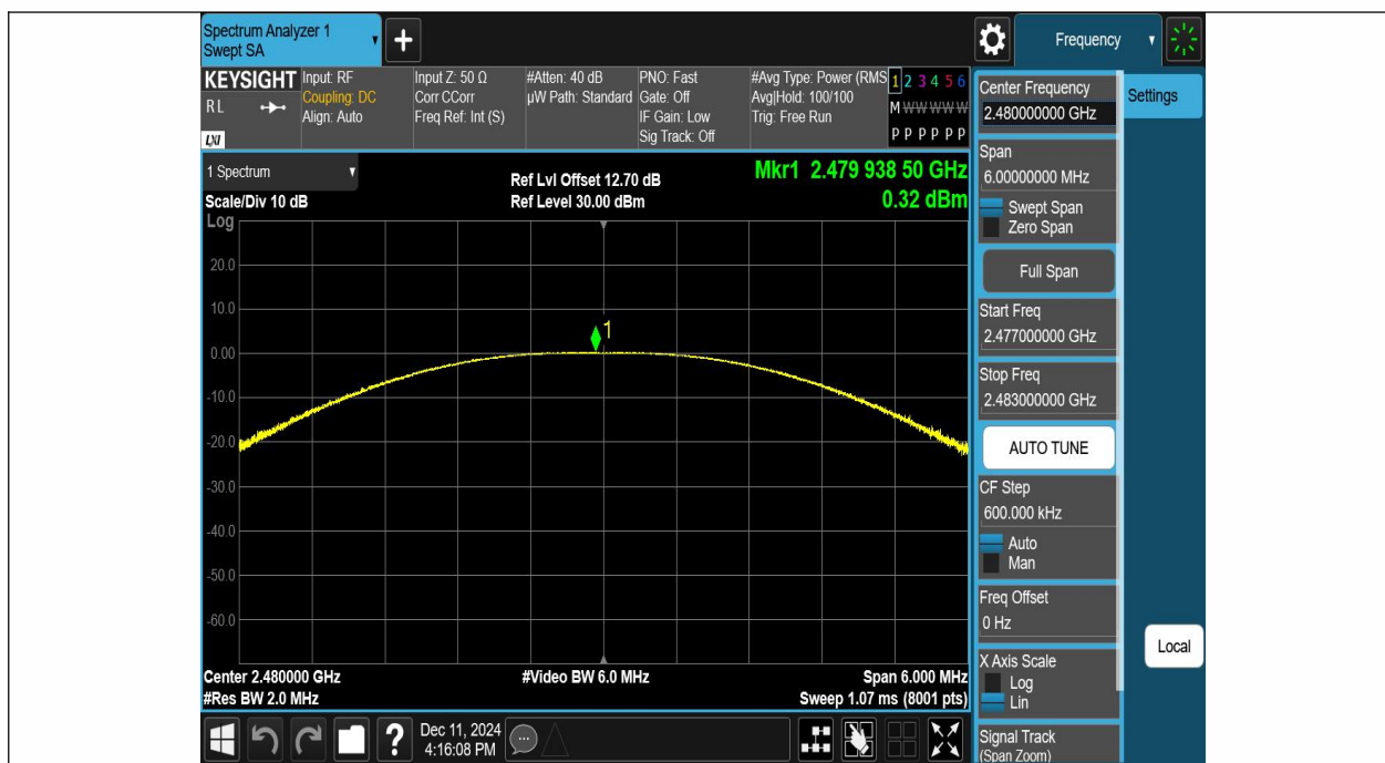
2.4G DTS MIMO-Ant1-2480-PASS
