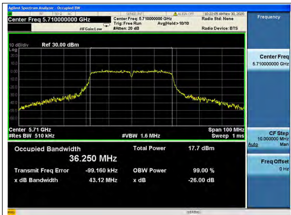
(Channel 142, 5710MHz, 802.11ac (VHT40))
