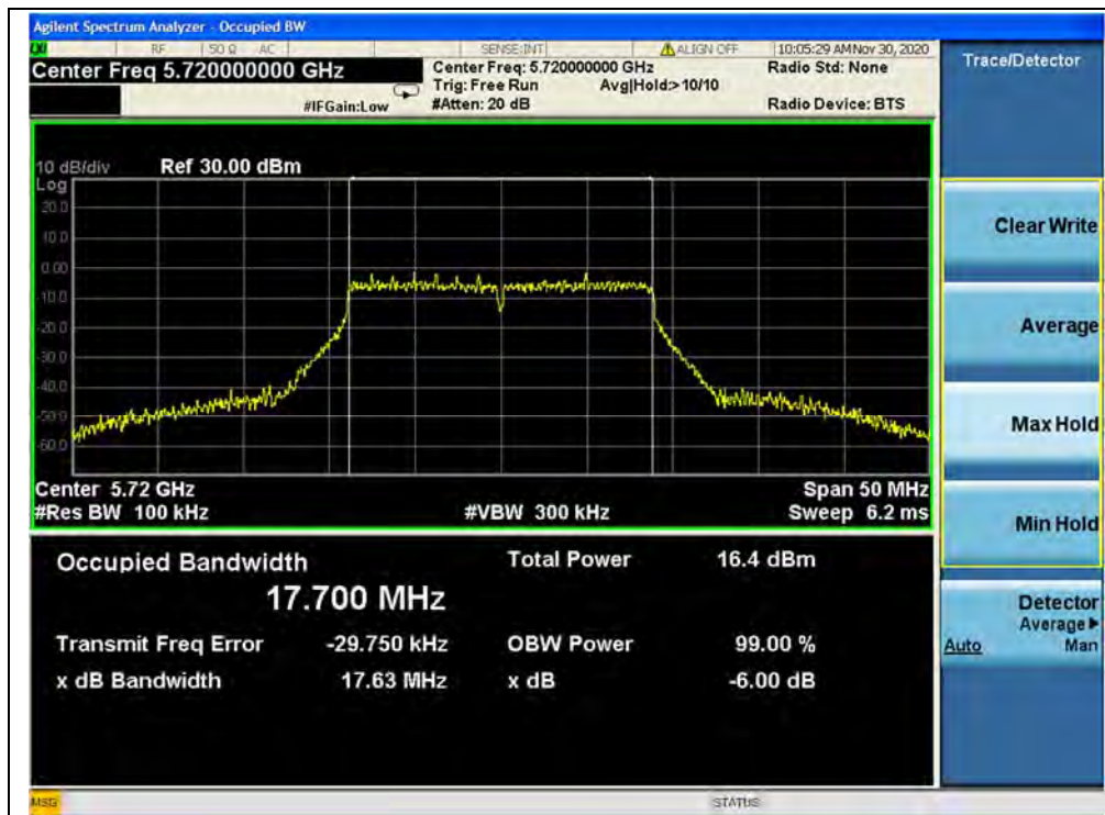
(Channel 144, 5720MHz, 802.11ac (VHT20))
