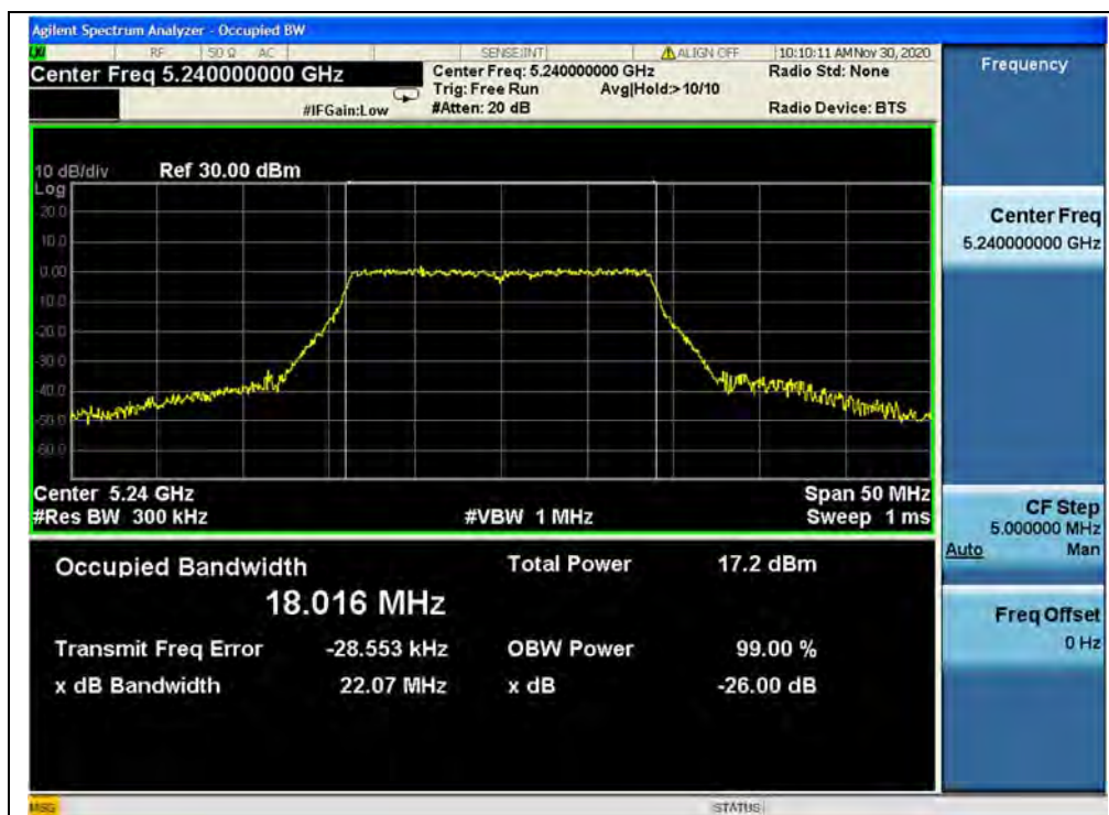
(Channel 48, 5240MHz, 802.11ac (VHT20))
