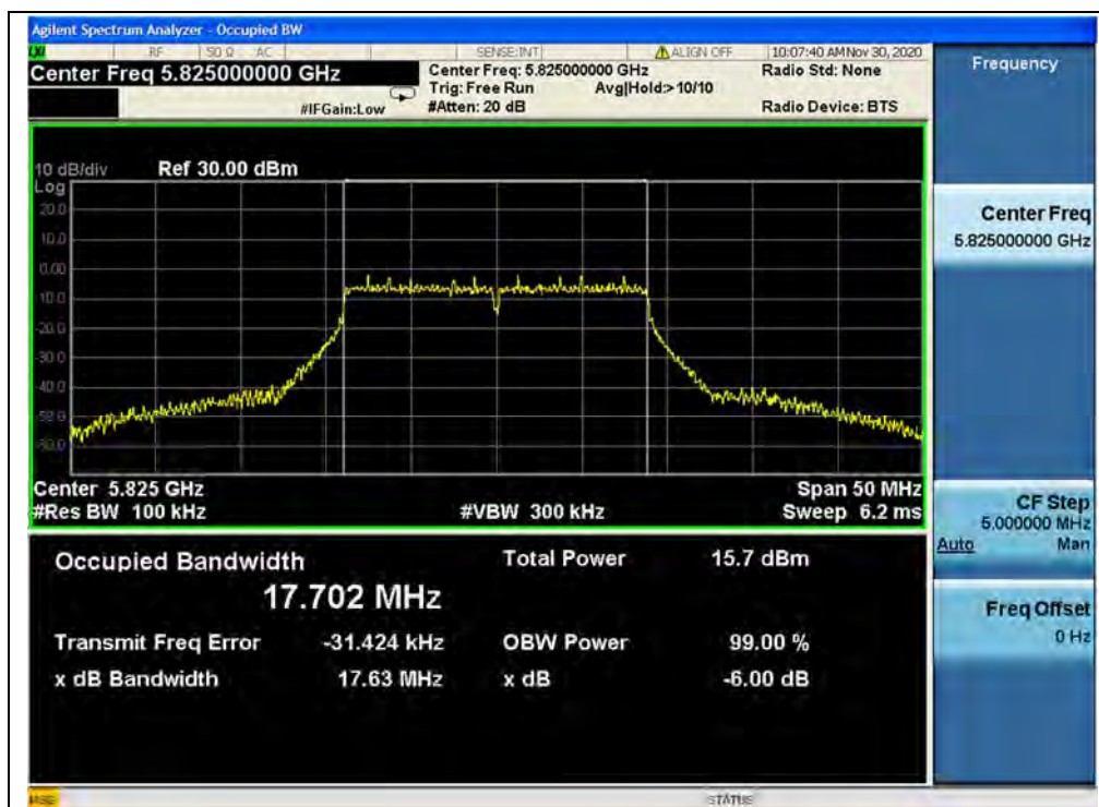
(Channel 165, 5825MHz, 802.11 ac (VHT20))
