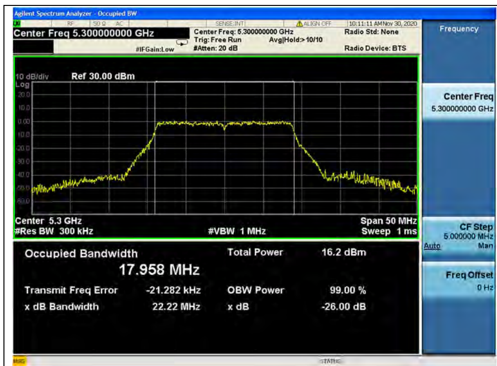
(Channel 60, 5300MHz, 802.11ac (VHT20))
