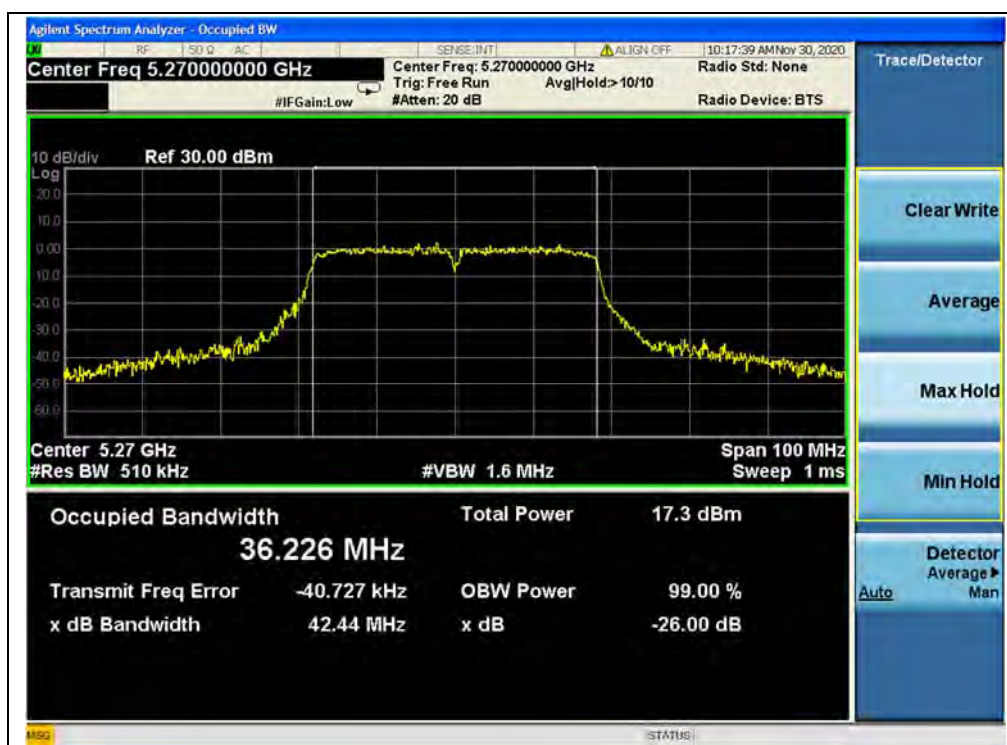
(Channel 54, 5270MHz, 802.11ac (VHT40))
