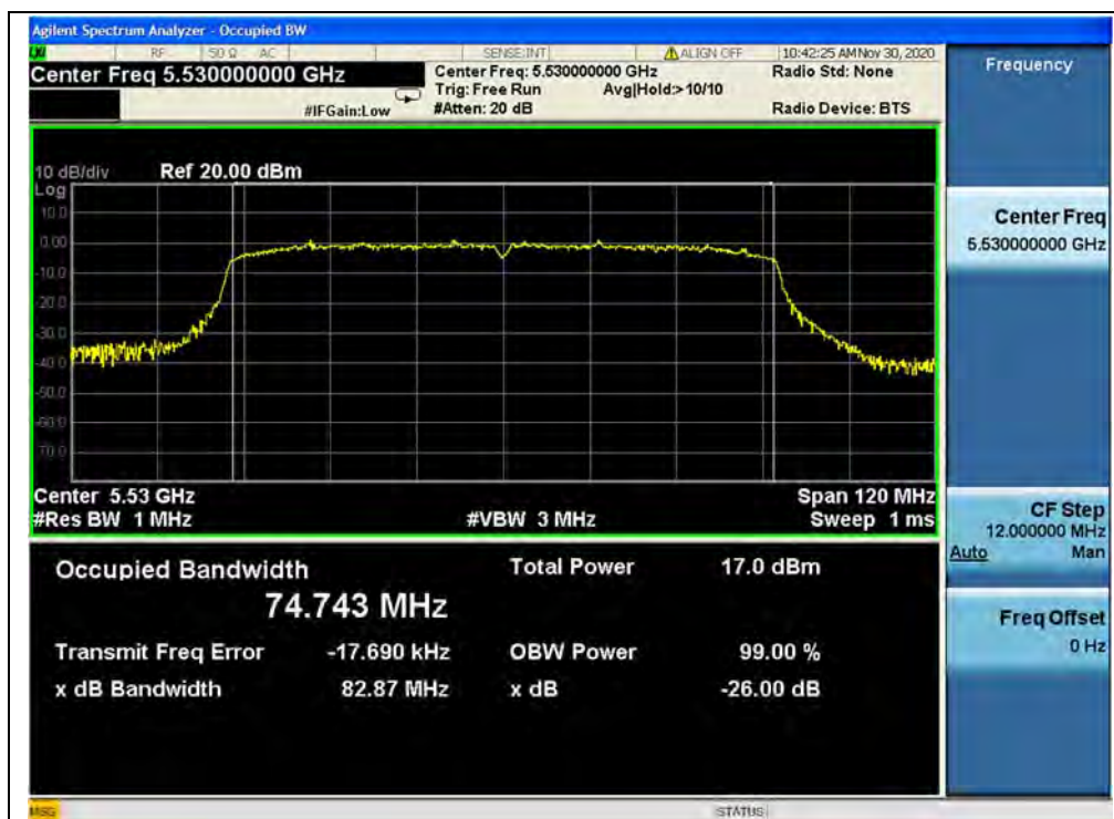
(Channel 106, 5530MHz, 802.11ac (VHT80))
