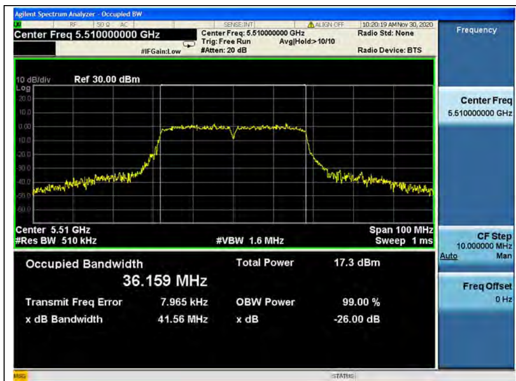
(Channel 102, 5510MHz, 802.11ac (VHT40))
