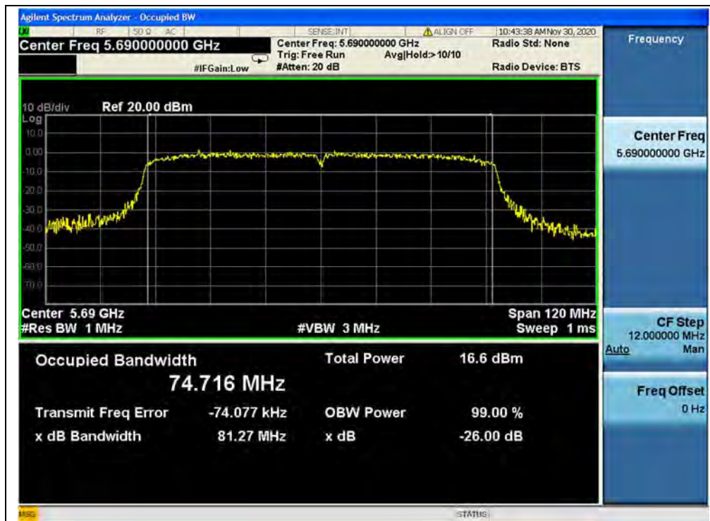
(Channel 138, 5690MHz, 802.11ac (VHT80))
