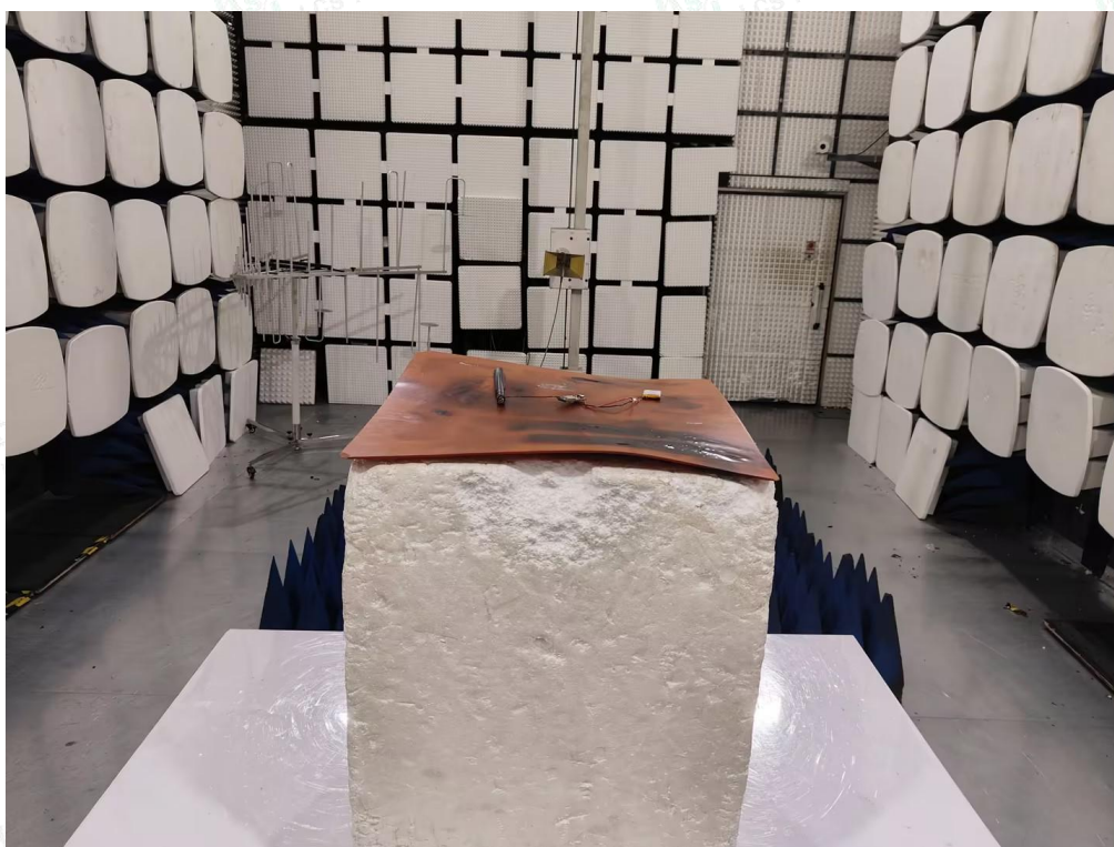
Radiated Emissions Measurement (Above 1GHz)
