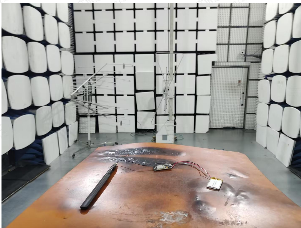
Radiated Emissions Measurement (Below 1GHz)
