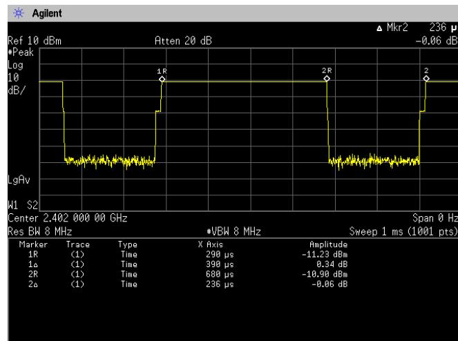
$$\text{Duty Cycle} = \text{Ton} / (\text{Ton} + \text{Toff}) = 390[\mu\text{s}] / (390[\mu\text{s}] + 236[\mu\text{s}]) = 62.3[\%]$$
