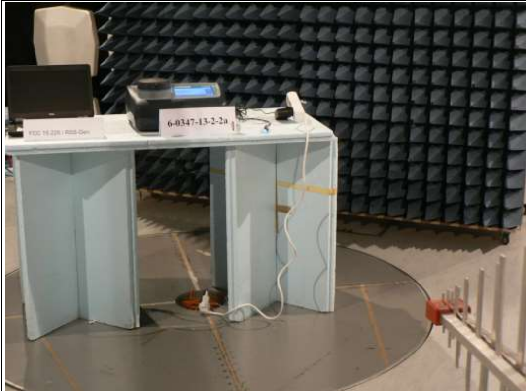
Photograph 3: Radiated measurements test set-up
