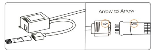
Step2: Connect the LED Controller with power supply.
