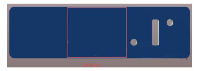
The label is attached to the bottom with a permanent adhesive.
