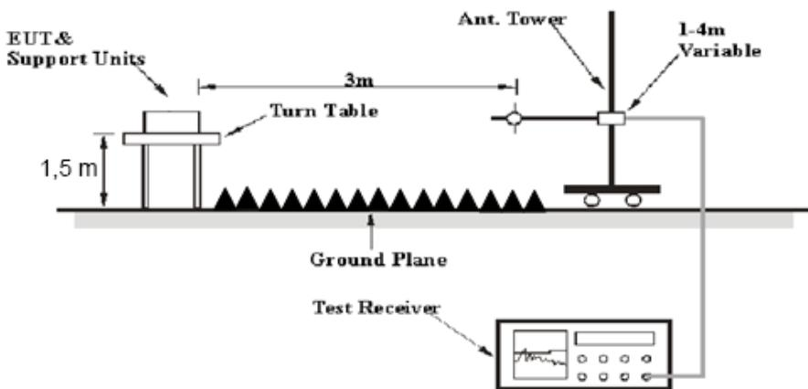
The radiated emission Below 1GHz tests were performed in the 3 meters chamber, above 1GHz tests were performed in the 3 meters chamber B, using the setup accordance with the ANSI C63.10-2013. The specification used was the FCC 15.209, and FCC 15.247 limits.
