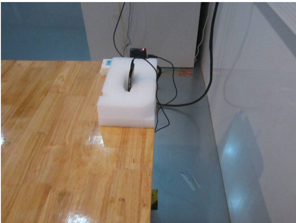
Conducted Emissions Test Setup Side View
