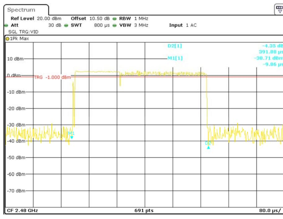
**Pulse time, Low Channel, 2DH3**
