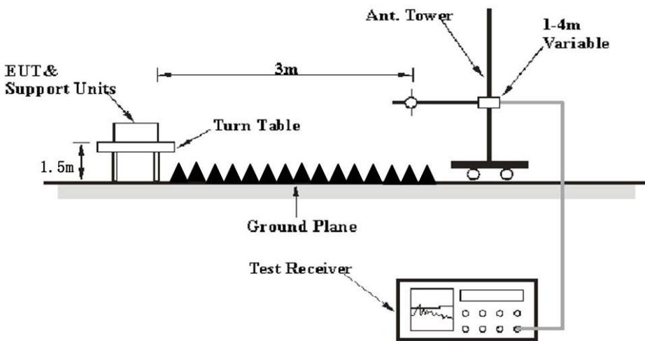
The radiated emission tests were performed in the 3 meters, using the setup accordance with the ANSI ANSI C63.10-2013. The specification used was the FCC 15.209 and FCC 15.247 limits.
