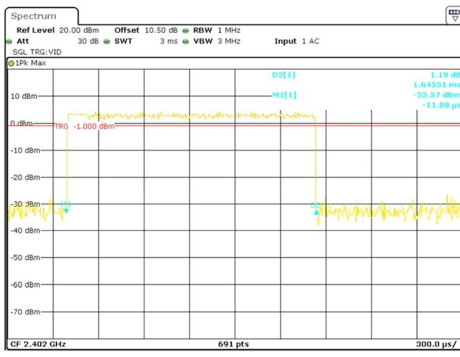
**Pulse time, Middle Channel, 3DH3**
