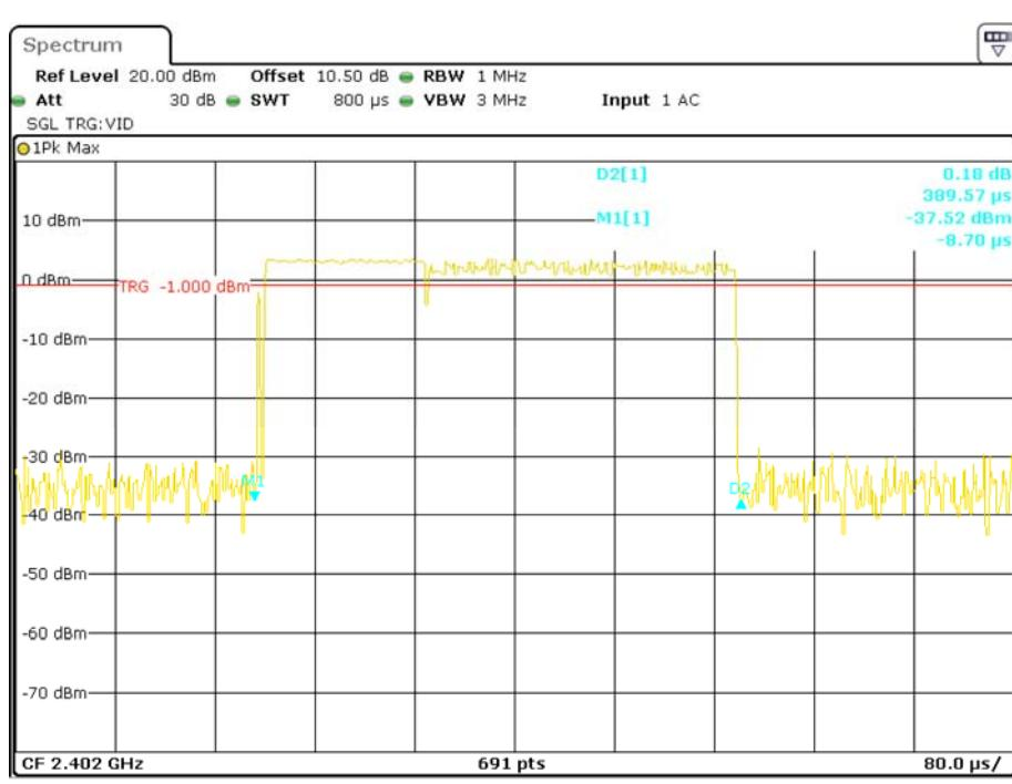
**Pulse time, Middle Channel, 2DH1**
