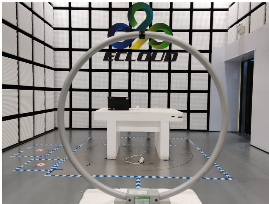
Fig. 1 Radiated emission setup photo(Below 30MHz)
