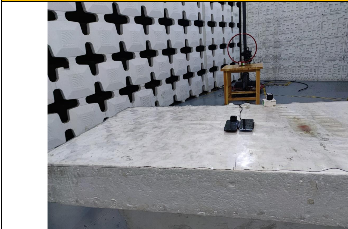
Radiated emission Test Setup (Below 30MHz)
