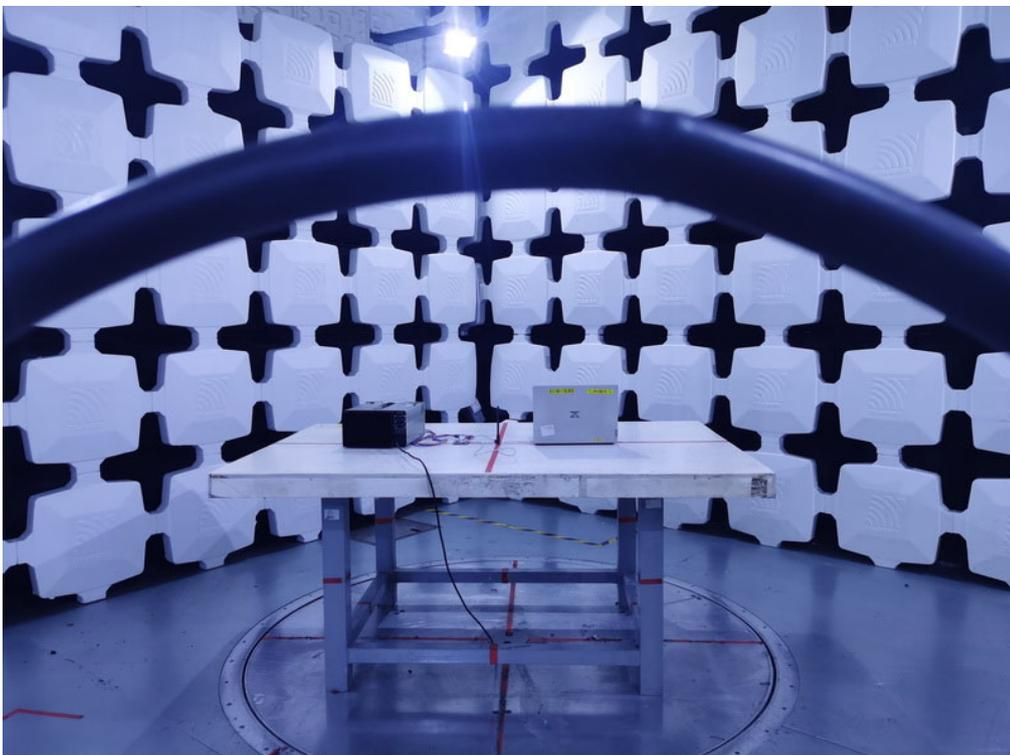
**Radiated Emissions Test Photos****30 MHz to 1 GHz**
