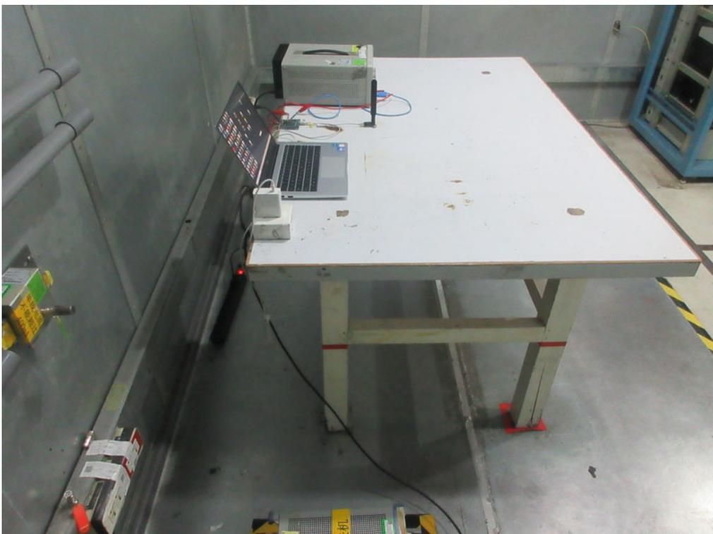
**Radiated Emissions Test Photos****9 kHz to 30 MHz**
