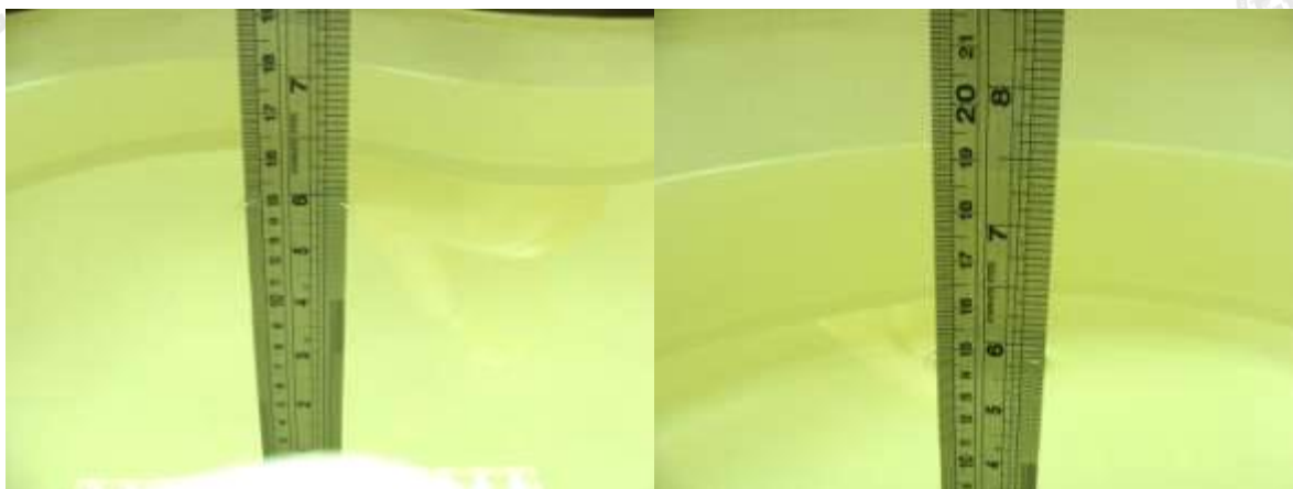
Photo of Liquid Height for Head SAR
