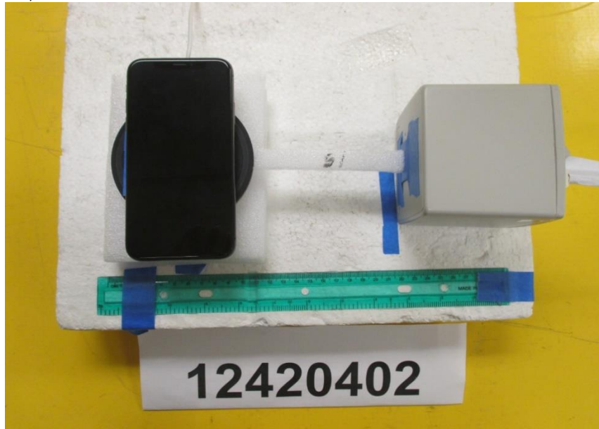
S1, RF EXPOSURE SETUP PHOTO
