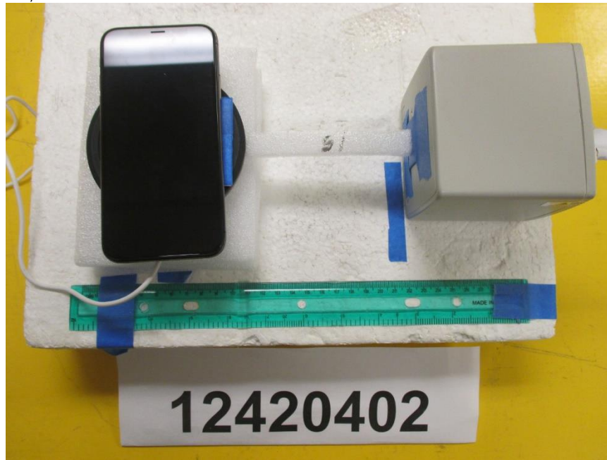
S3, RF EXPOSURE SETUP PHOTO
