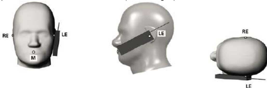
Fig. 11.3 Illustration for Cheek Position
