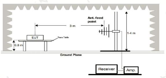
3. Radiated Emission Test-Up Frequency Above 1GHz
