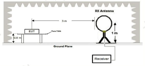
2. Radiated Emission Test-Up Frequency 30MHz~1GHz
