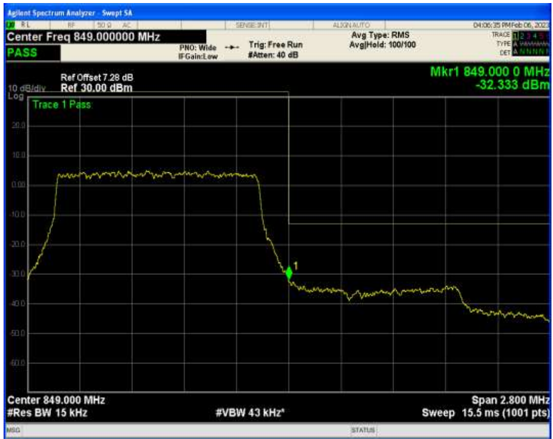
Band5 QPSK BW=10MHz Channel=20450 RB Size=50 Position=#0
