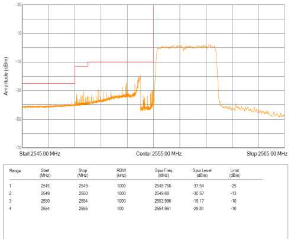
Band41(2555-2655) QPSK BW=5MHz Channel=41215 RB Size=25 Position=#0
