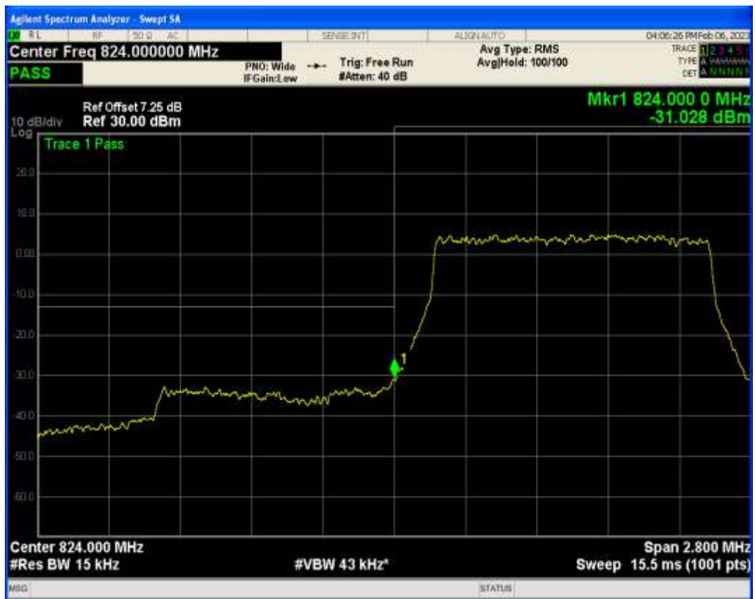
Band5 QPSK BW=1.4MHz Channel=20643 RB Size=6 Position=#0
