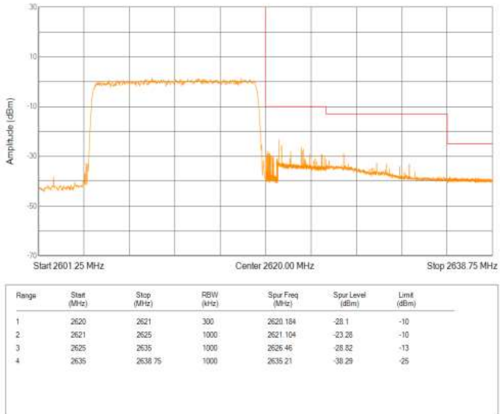
Band38 16QAM BW=20MHz Channel=37850 RB Size=100 Position=#0
