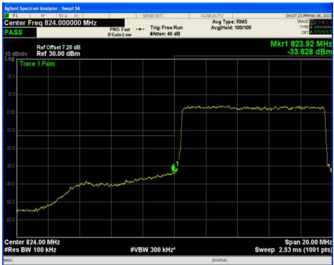
Band5 QPSK BW=10MHz Channel=20600 RB Size=50 Position=#0
