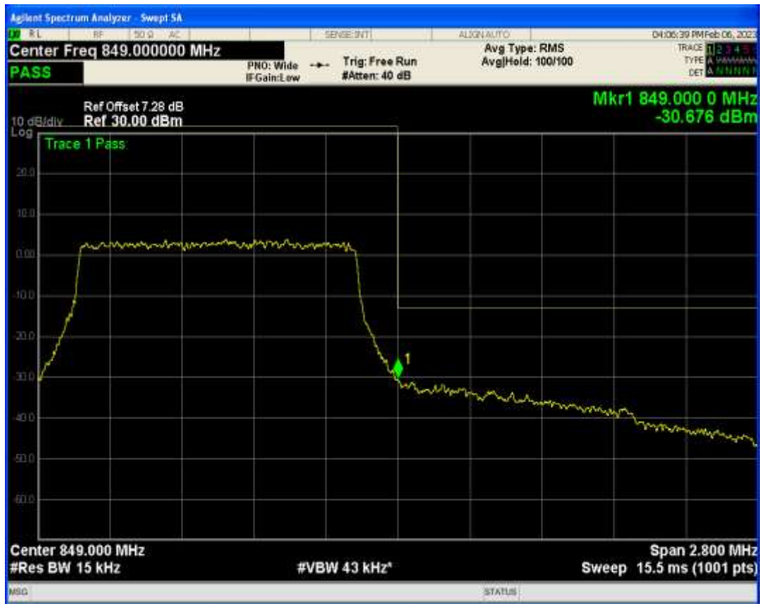
Band5 16QAM BW=10MHz Channel=20450 RB Size=50 Position=#0
