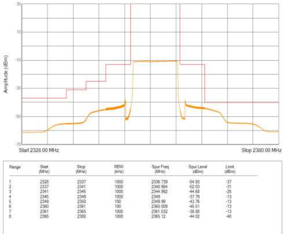
Band40(2350-2360) QPSK BW=5MHz Channel=39175 RB Size=25 Position=#0
