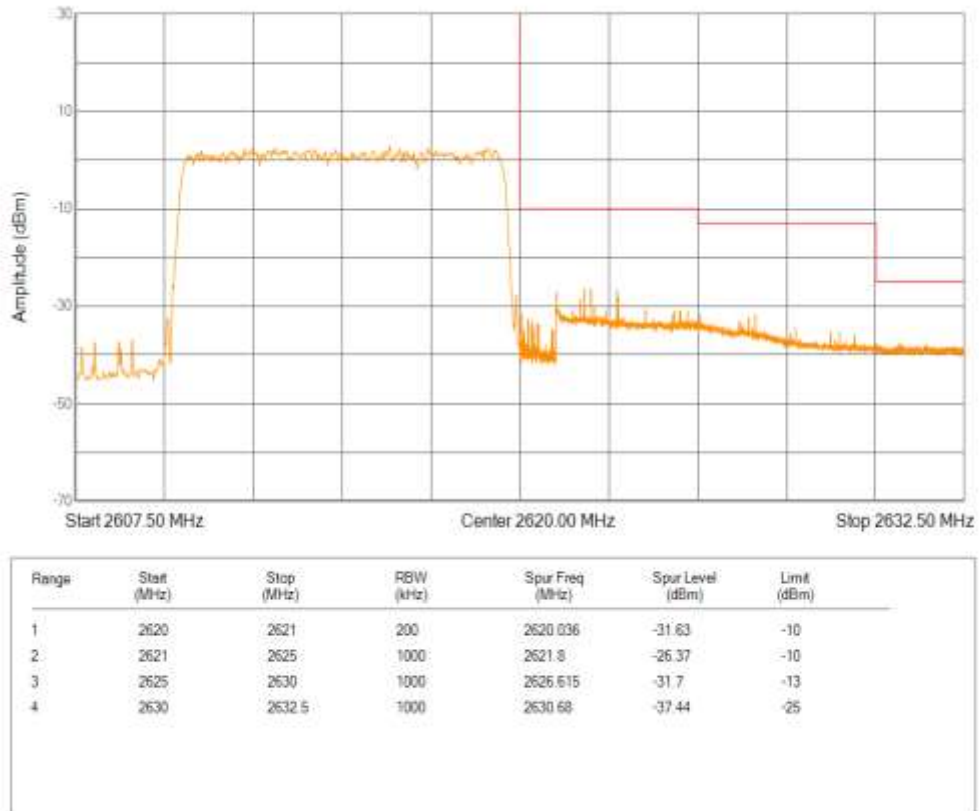
Band38 QPSK BW=15MHz Channel=37825 RB Size=75 Position=#0
