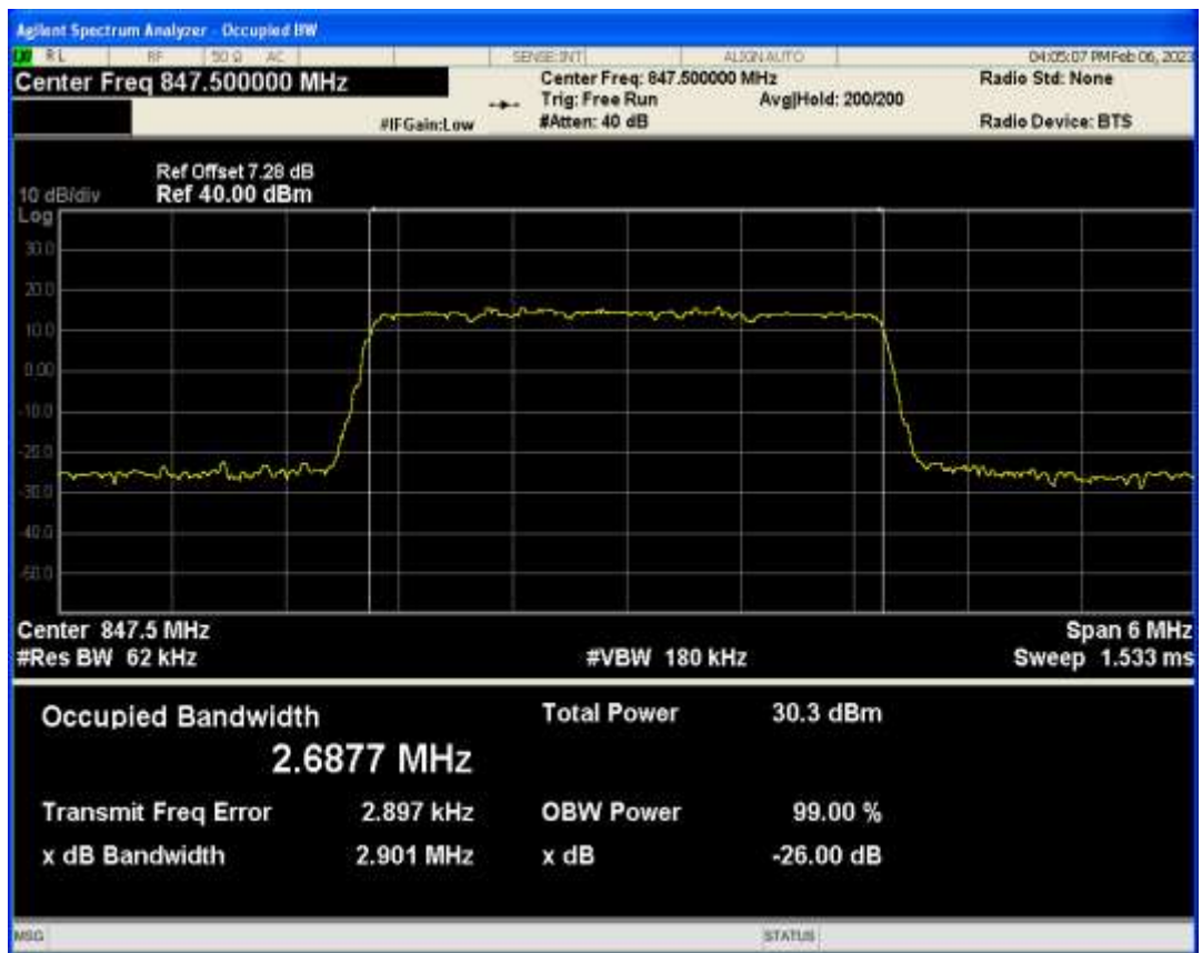
Band5 QPSK BW=5MHz Channel=20425 RB Size=25 Position=#0
