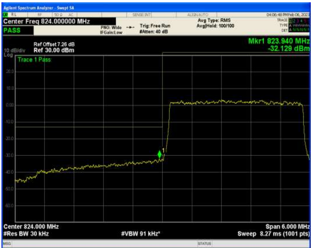
Band5 16QAM BW=3MHz Channel=20635 RB Size=15 Position=#0
