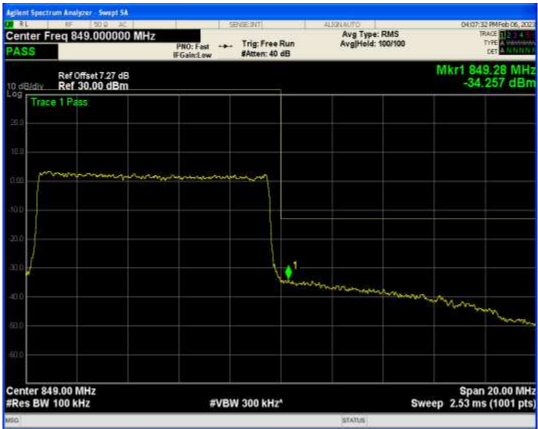
Band5 16QAM BW=3MHz Channel=20415 RB Size=15 Position=#0
