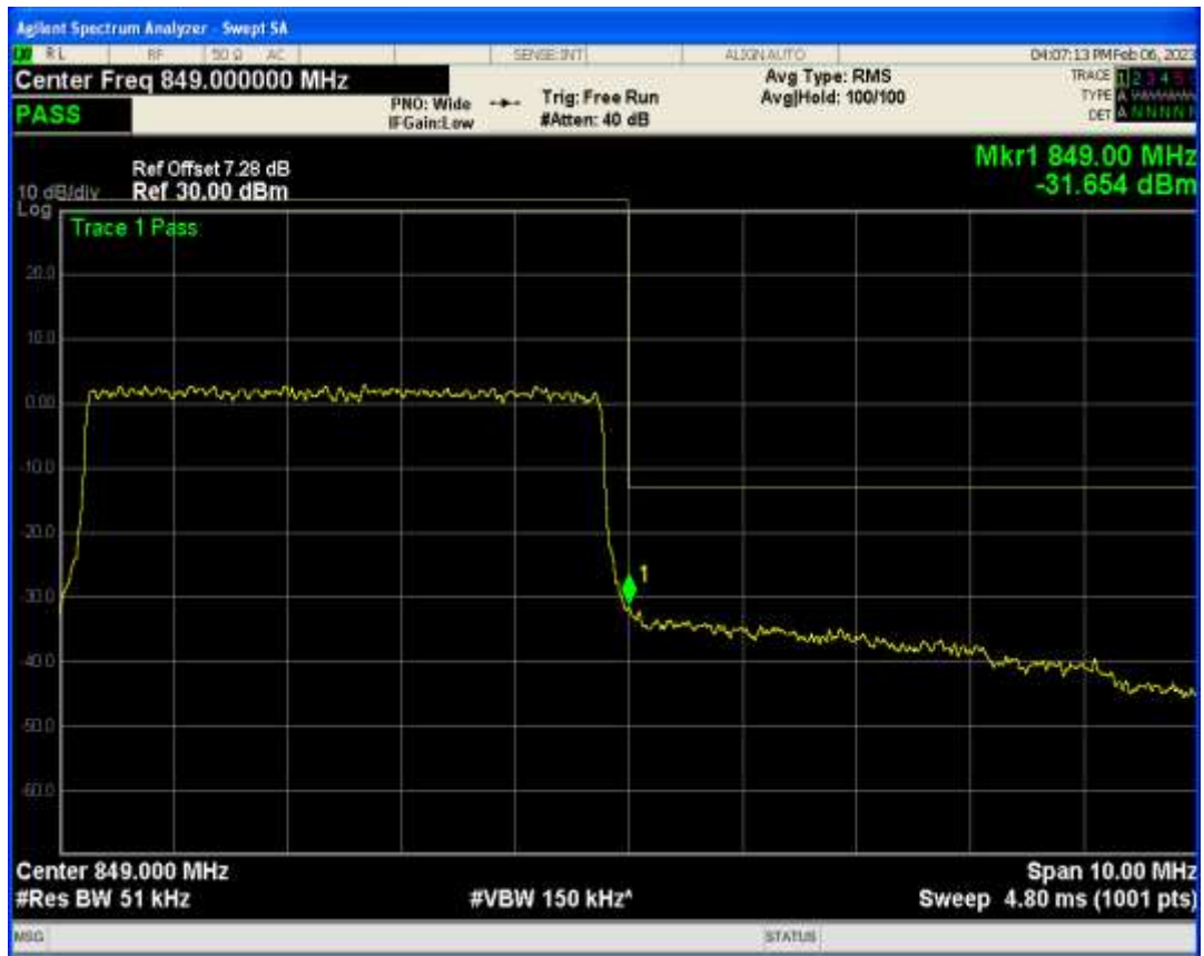
Band5 QPSK BW=1.4MHz Channel=20407 RB Size=6 Position=#0
