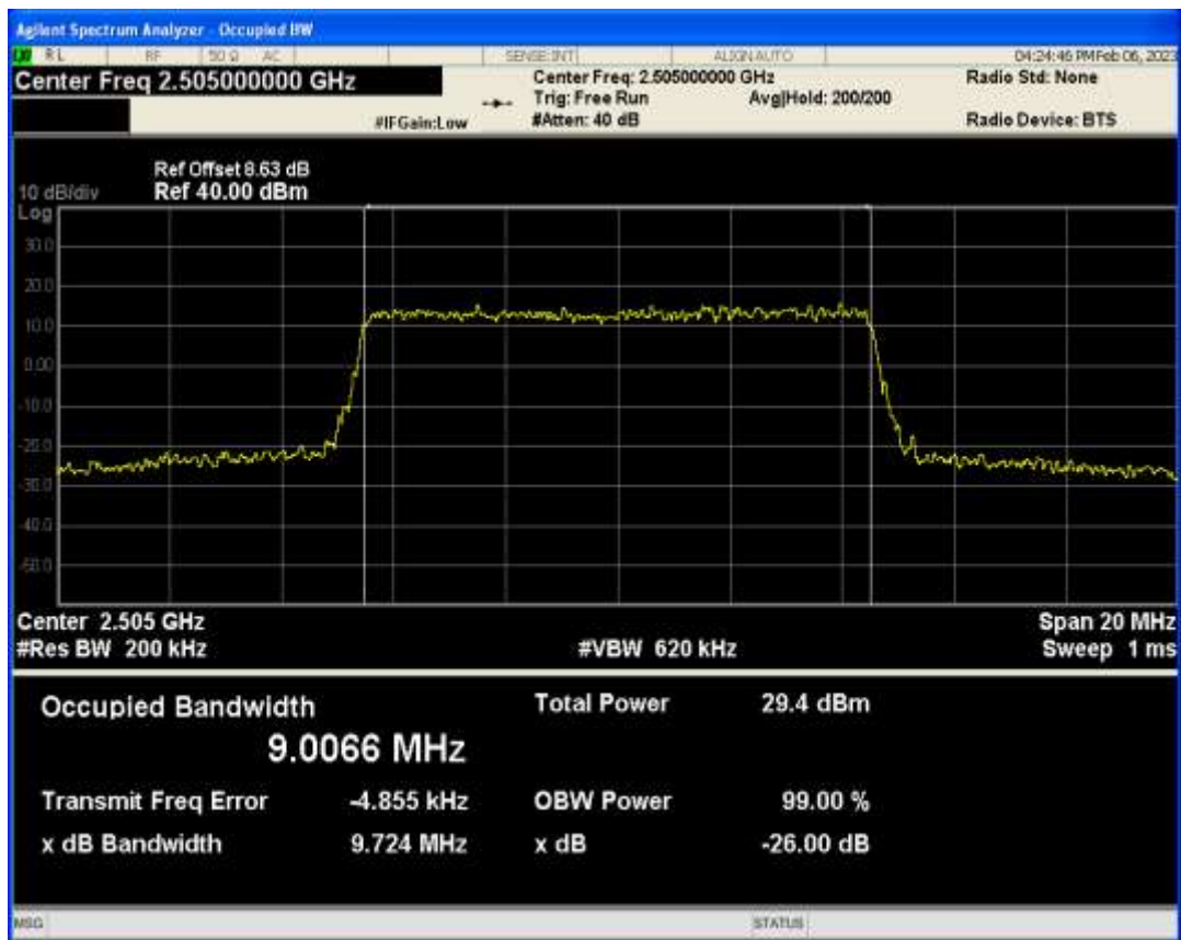
Band7 QPSK BW=10MHz Channel=21100 RB Size=50 Position=#0
