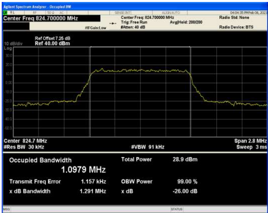
Band5 16QAM BW=1.4MHz Channel=20525 RB Size=6 Position=#0
