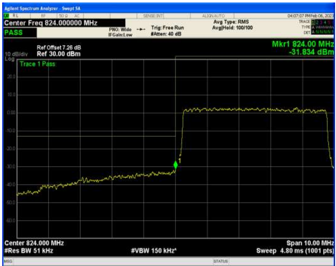
Band5 16QAM BW=5MHz Channel=20625 RB Size=25 Position=#0
