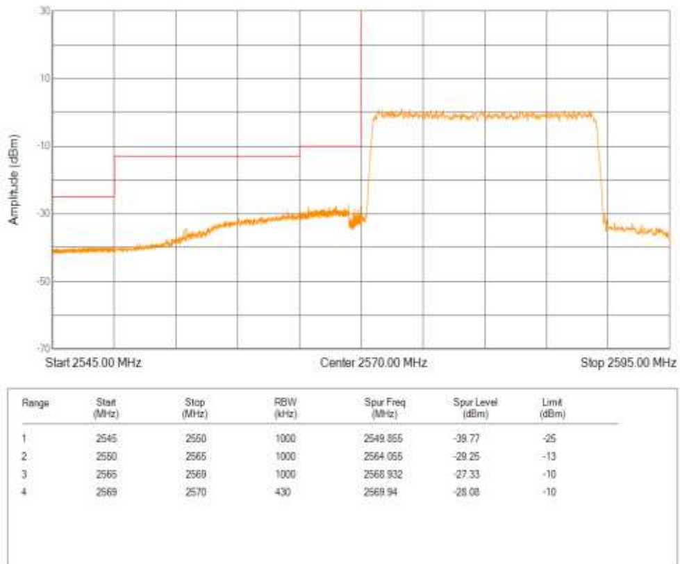
Band38 16QAM BW=20MHz Channel=38150 RB Size=100 Position=#0
