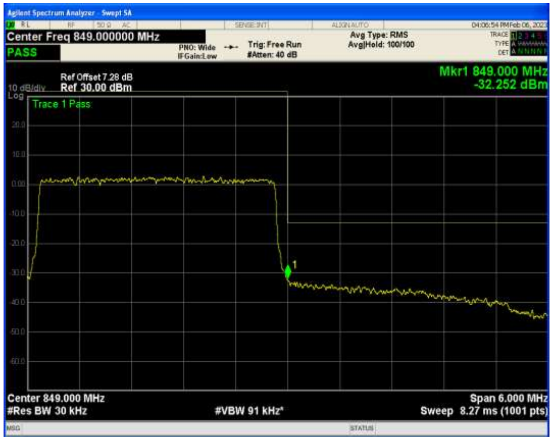
Band5 16QAM BW=5MHz Channel=20425 RB Size=25 Position=#0
