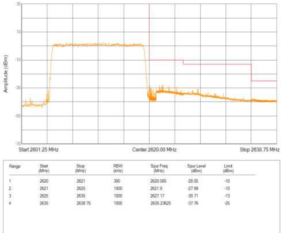
Band38 QPSK BW=20MHz Channel=37850 RB Size=100 Position=#0
