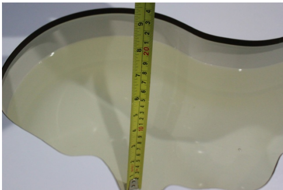
Liquid depth in the head phantom (2450MHz)
