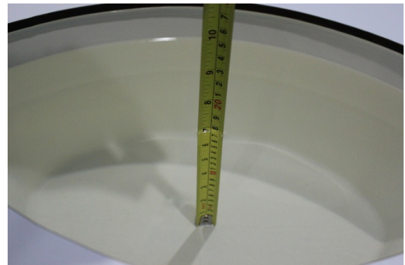
Liquid depth in the body phantom (2450MHz)
