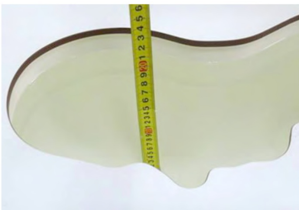
Liquid depth in the head phantom (1900MHz)
