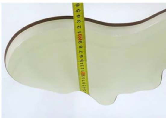
Liquid depth in the head phantom (1750MHz)
