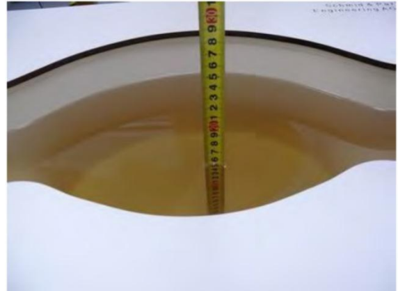
Liquid depth in the body phantom (750MHz)
