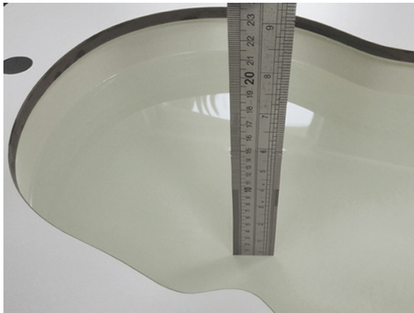
Liquid depth in the head phantom (2450MHz)
