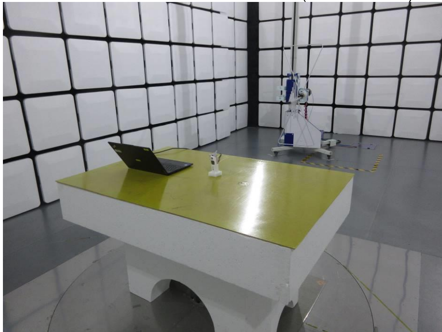
RADIATED RF MEASUREMENT SETUP (30MHz ~ 1 GHz)
