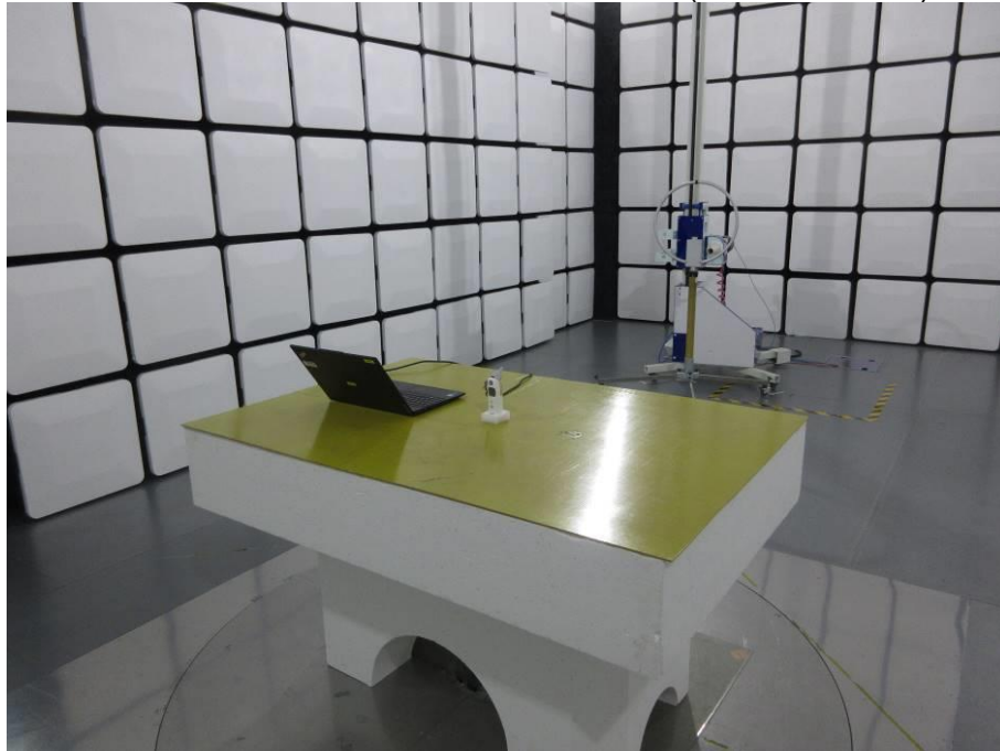
RADIATED RF MEASUREMENT SETUP (9kHz ~ 30 MHz)
