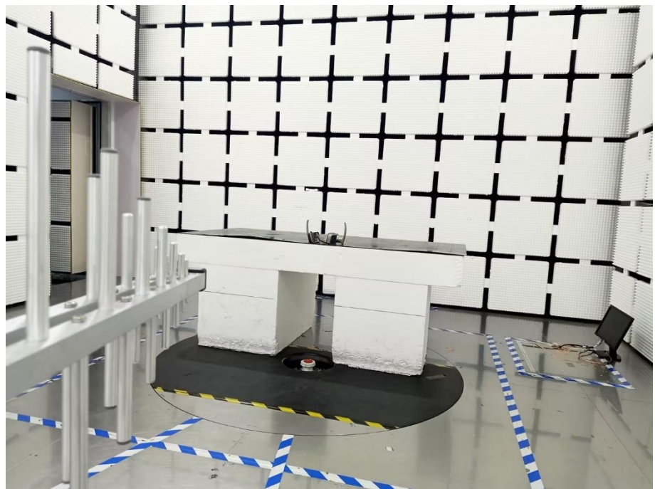
Radiation Emission Test Setup (30MHz to 1GHz)
