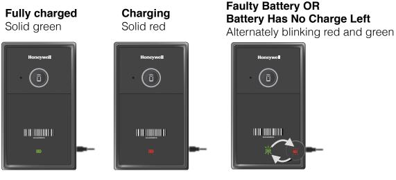
If Battery has no charge left, the Gateway needs 15-20 minutes to precharge, before the battery starts charging normally.
