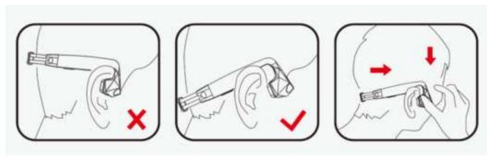
Bone conduction earphones do not need to be inserted into or cover the ears, but the vibration unit (commonly known as: vibrator or speaker) is attached to the temporal bone protrusion in front of the human ear. It will be very comfortable to wear correctly and will not cause any burden on the ear and neck
