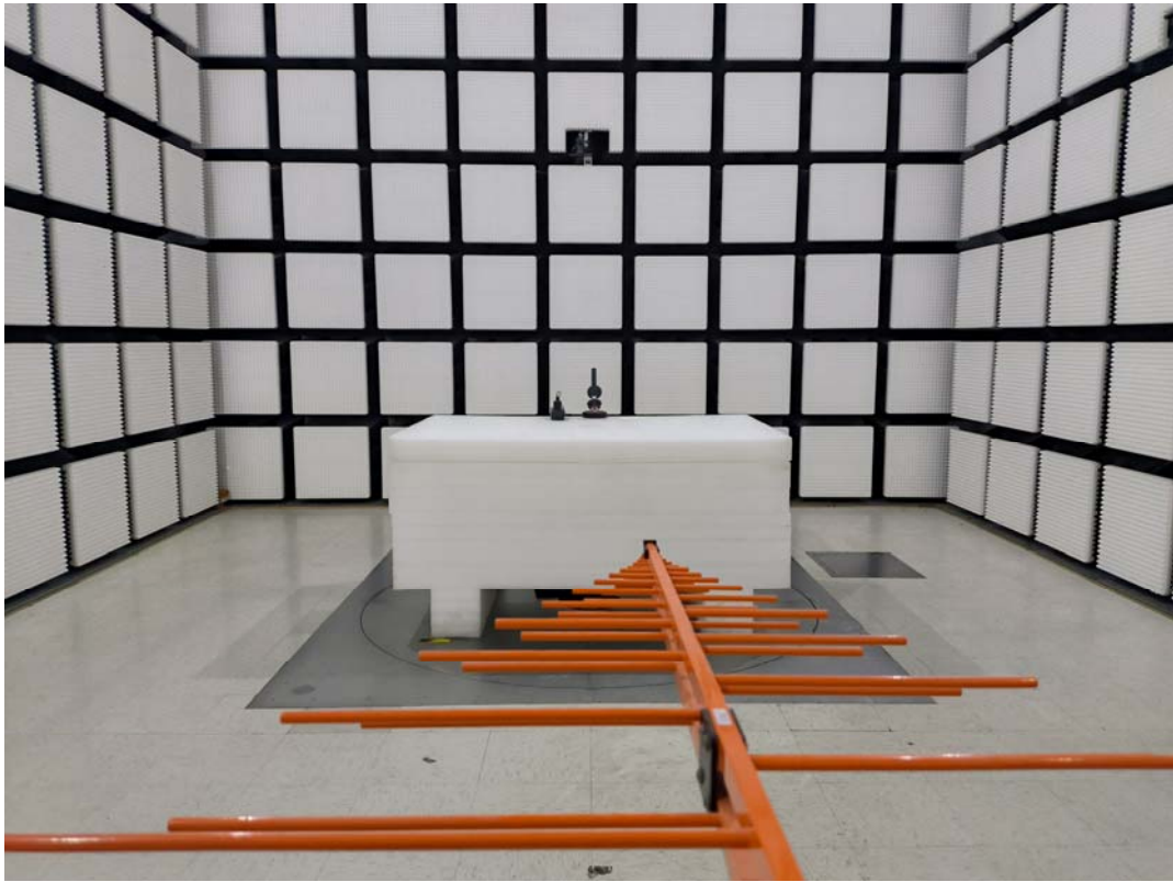
Radiated Emission Below 1GHz rear View -M2
