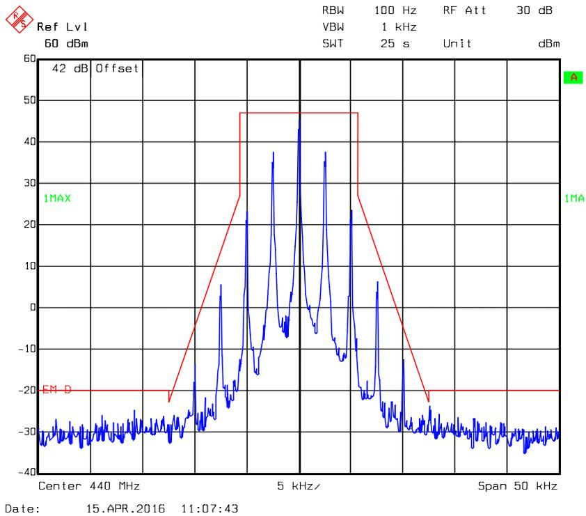
**Occupied Bandwidth -12.5kHz, 440 MHz, Middle Power Level**
