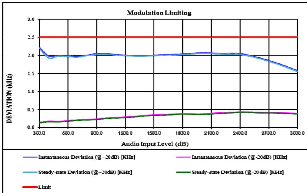
Carrier Frequency: 155 MHz, Channel Spacing = 6.25 kHz
