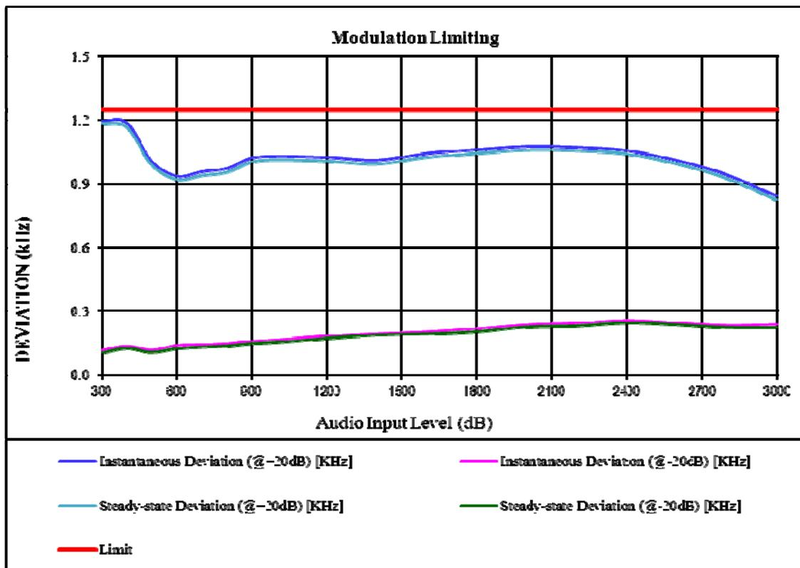
Carrier Frequency: 440 MHz, Channel Spacing =12.5 kHz
