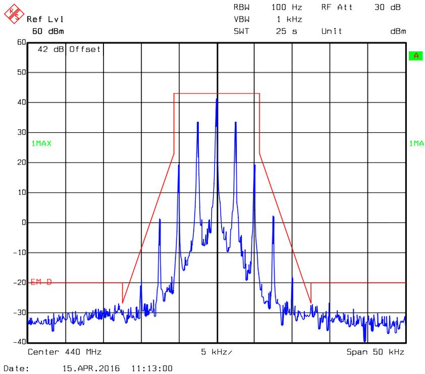
**Occupied Bandwidth – 12.5kHz, 440 MHz, Low Power Level**
