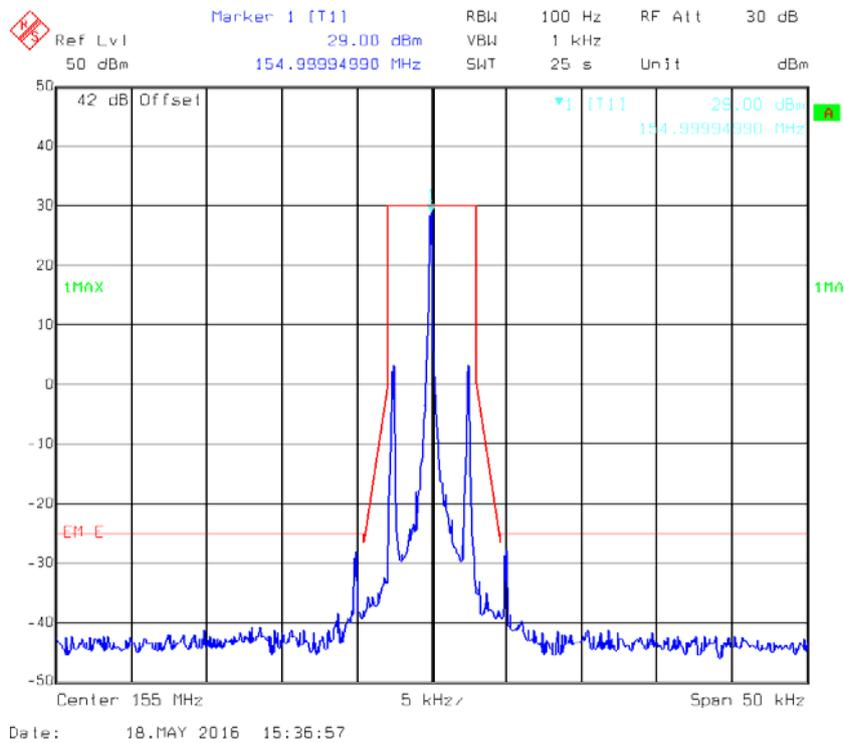
**Occupied Bandwidth –12.5kHz, 155 MHz, High Power Level**
