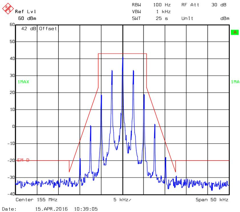
**Occupied Bandwidth – 12.5kHz, 155 MHz, Low Power Level**
