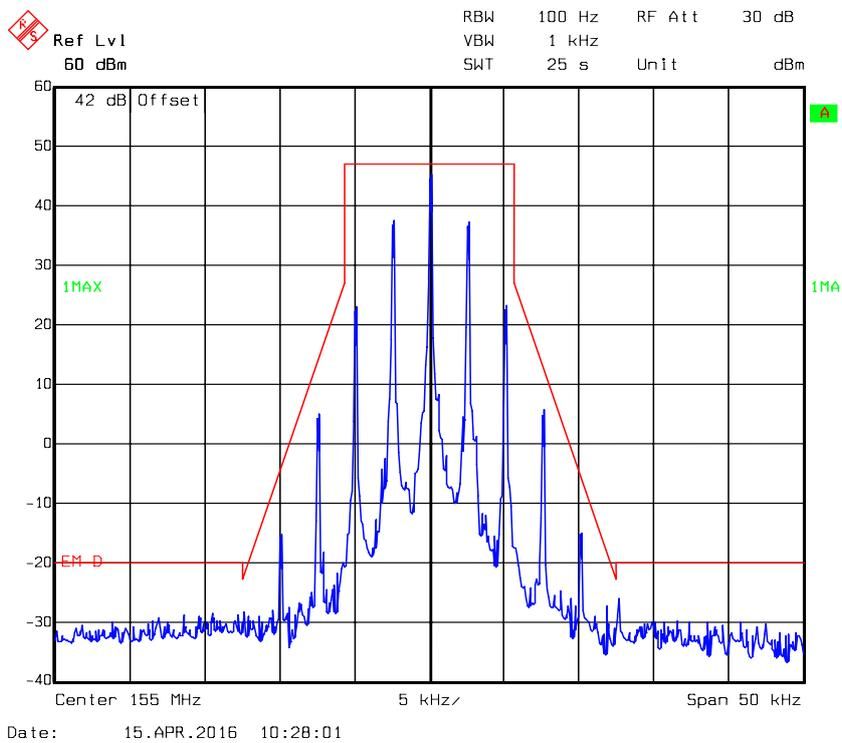
**Occupied Bandwidth -12.5kHz, 155 MHz, Middle Power Level**
