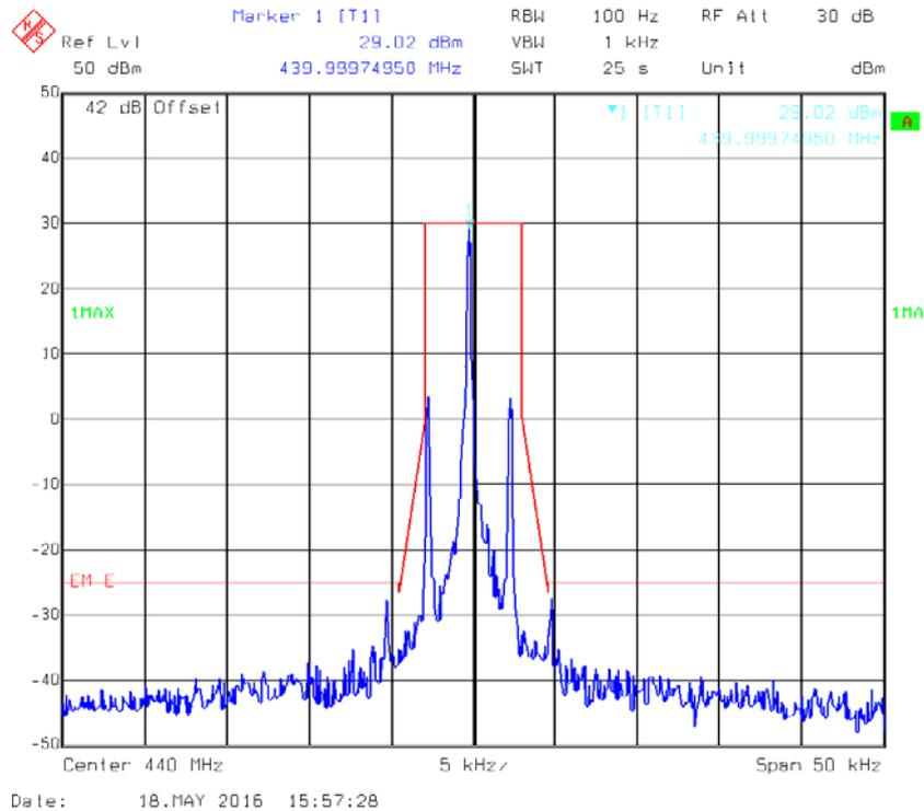
**Occupied Bandwidth -12.5kHz, 440 MHz, High Power Level**
