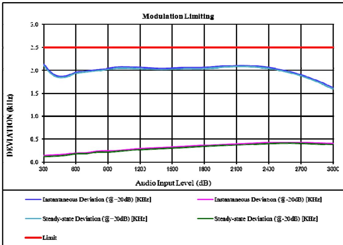
Carrier Frequency: 440 MHz, Channel Spacing =6.25 kHz
