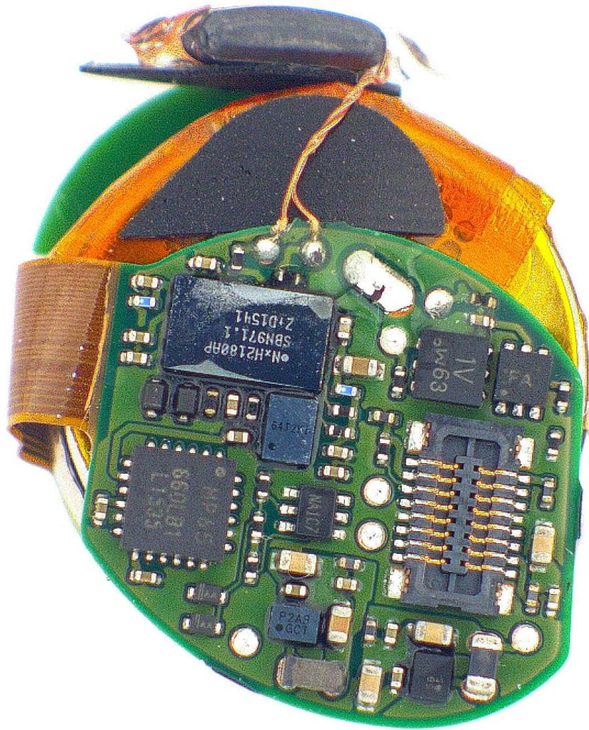
PC board top view (NFMI antennal on top)
