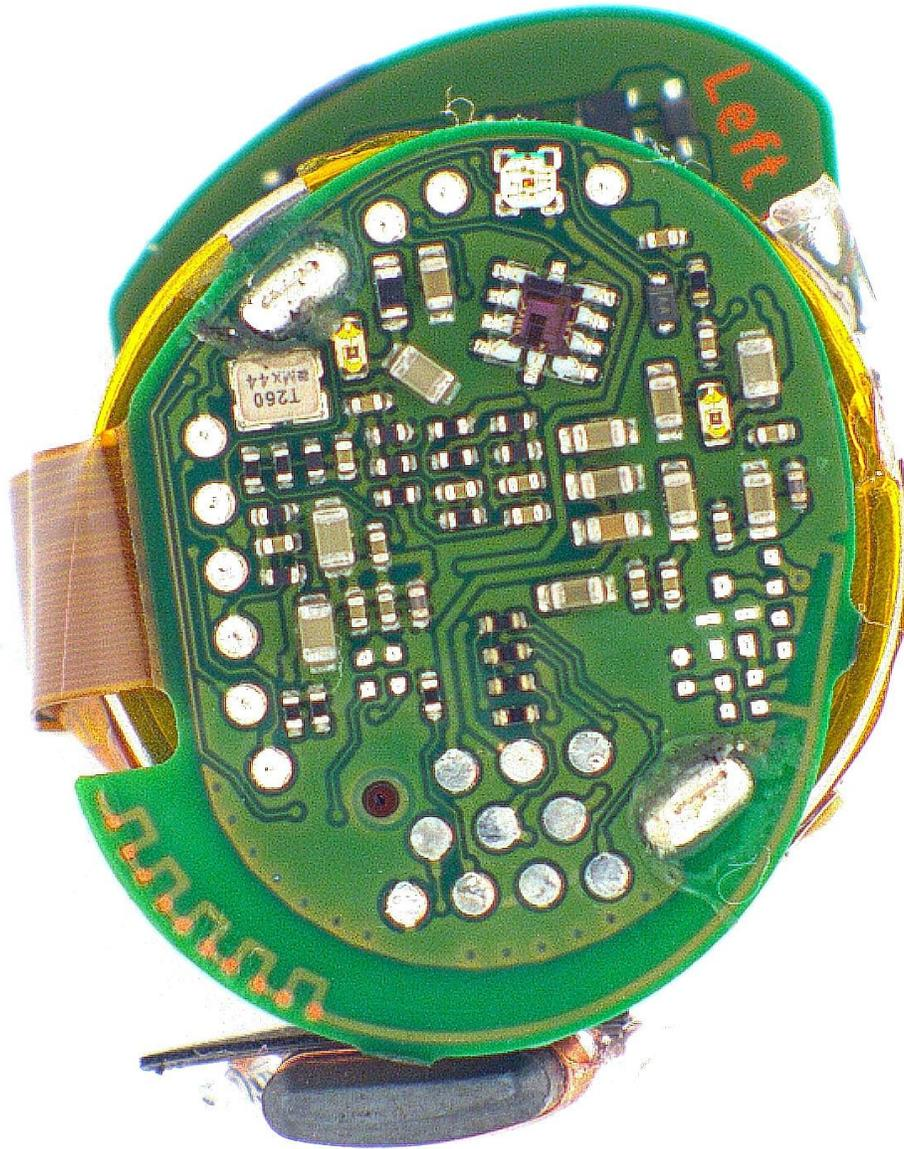
PC board bottom view (NFMI antenna on bottom)
