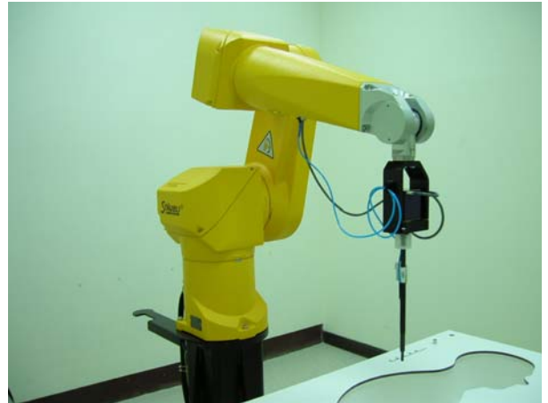
Fig. 5.2 Probe setup on robot
