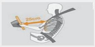
The minimum distance between the driver and the steering wheel
