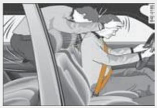
The rear passenger seat belt fastened will be thrown forward
