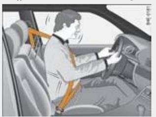
The driver who has fastened his seat belt will be pulled back by the properly fastened seat belt at sudden braking.
