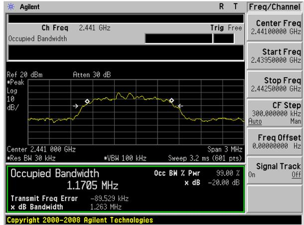
20dB Bandwidth plot on channel 78 (1Mbps)
