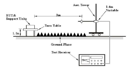
The radiated emission tests were performed in the 3 meters test site, using the setup accordance with the ANSI C63.10-2013 & RSS-Gen. The specification used was the FCC 15.209, and FCC 15.247 & RSS-Gen limits.
