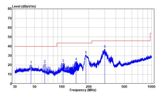
Site : chamber Condition: 3m HORIZONTAL Job No. : SZNS220313-08566E-RF Test Mode: 2.4G WIFI
