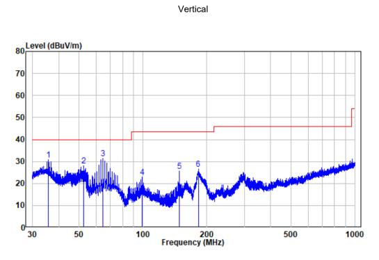
Site : chamber Condition: 3m VERTICAL Job No. : SZNS220313-08566E-RF Test Mode: 2.4G WIFI
