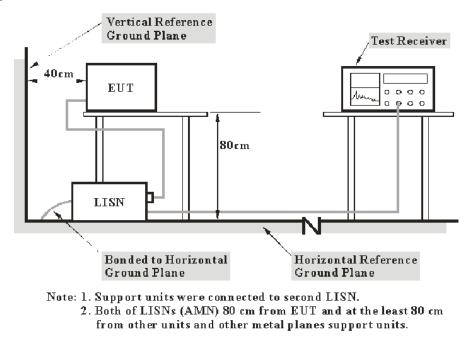
The setup of EUT is according with per ANSI C63.10-2013 measurement procedure. The specification used was with the FCC Part 15.207 & RSS-247/RSS-Gen limits.
