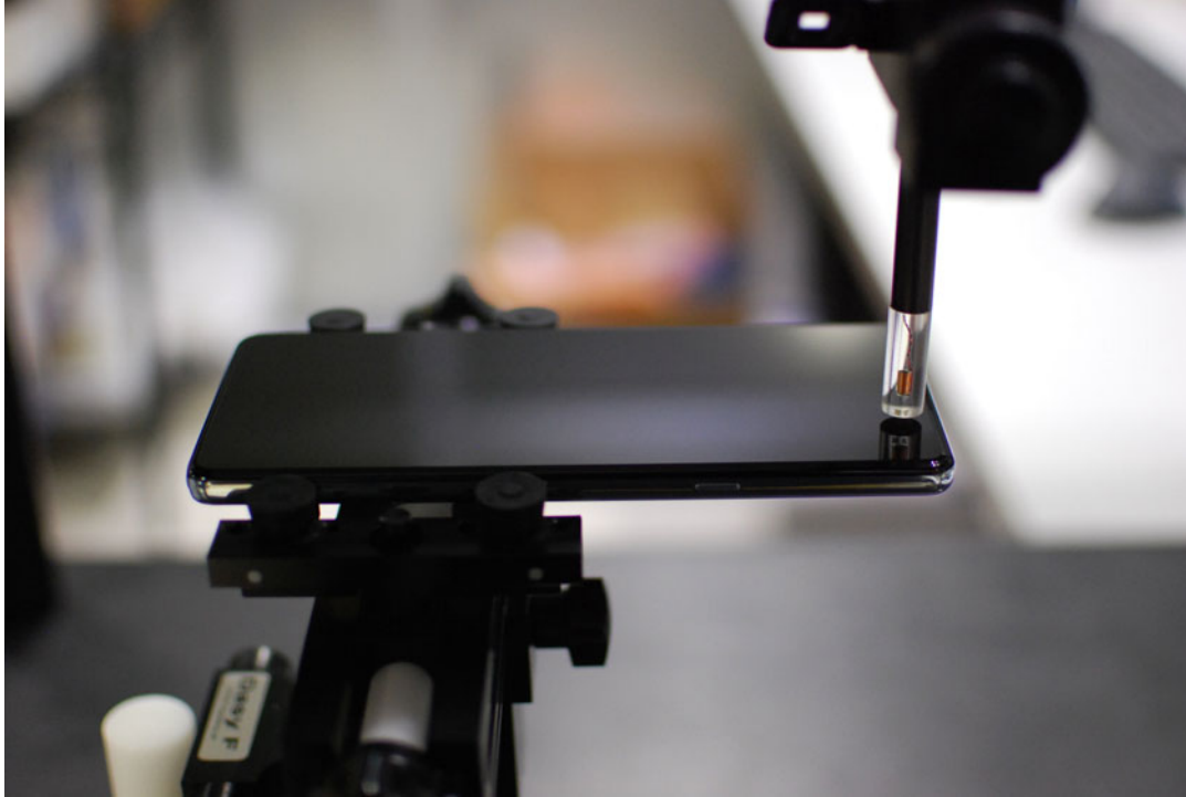
Figure 16-1 Test Setup for Wireless Device
