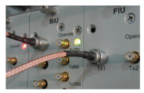
Figure 24 BTS QMA Coaxial Cable Connection
