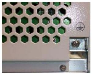
Figure 22Host Unit Grounding Stud
