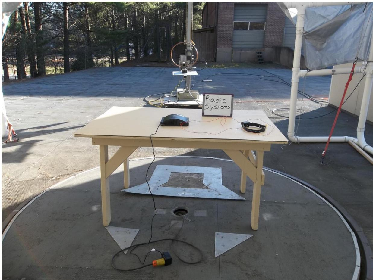
**Figure 2. Radiated Emissions Test Setup (below 30 MHz)**
