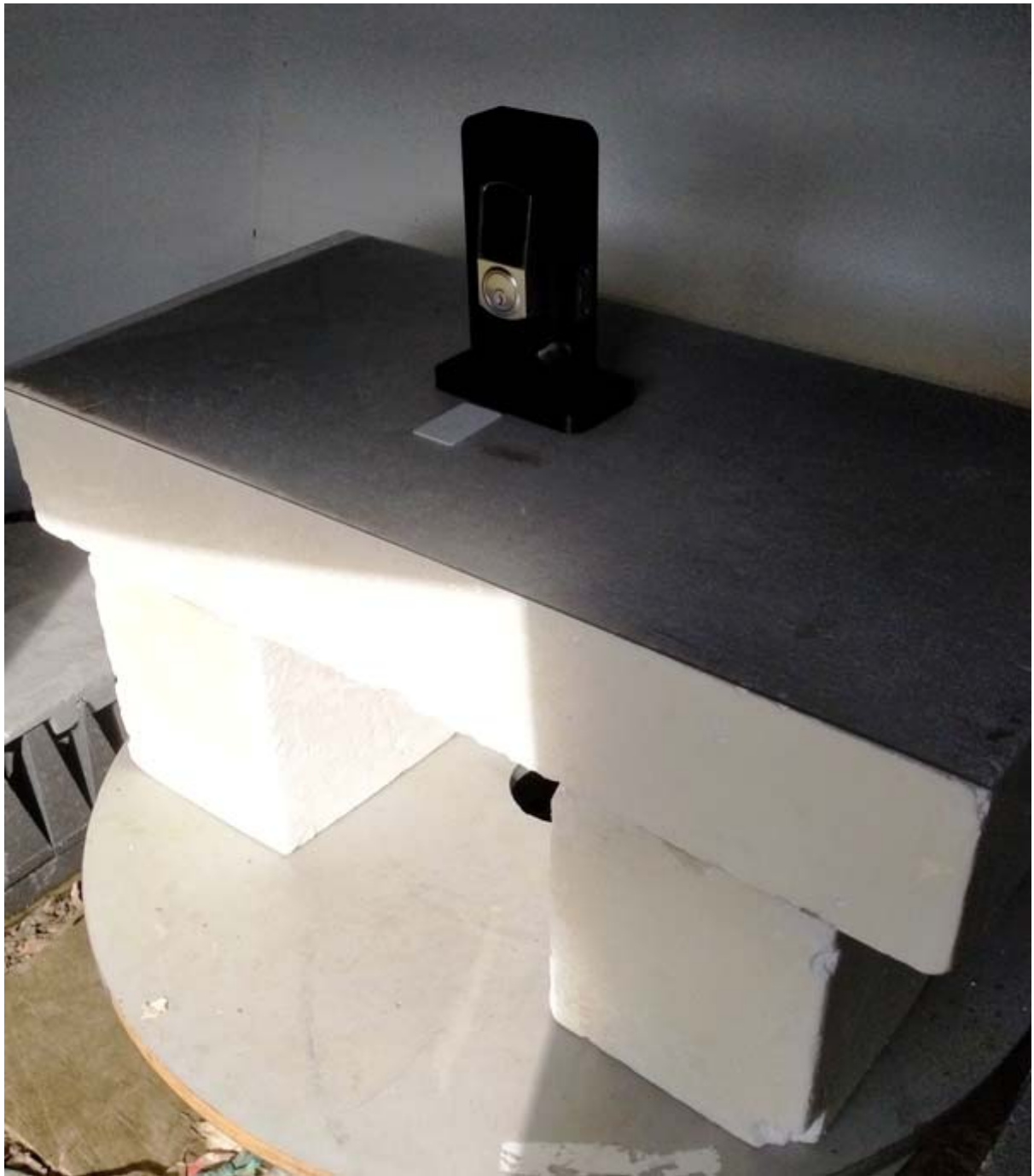
Test Set Up at 80 cm above the ground plane
