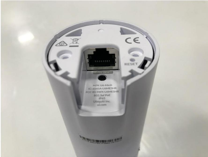
**Photograph 7: Bottom View Close-Up Showing Ethernet Port**
