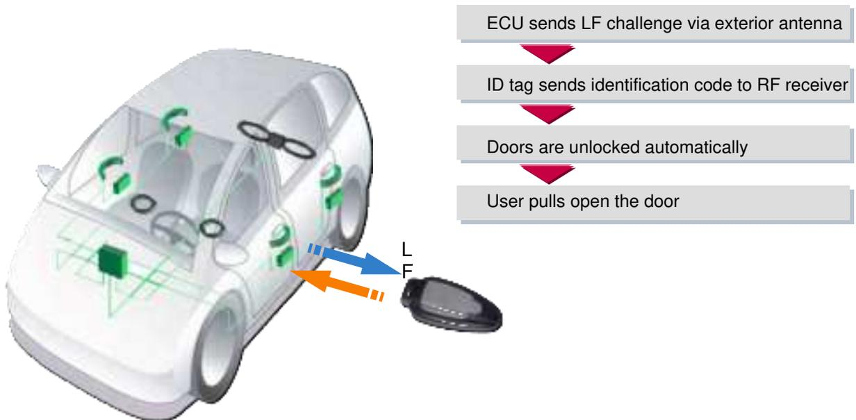
**Figure 1: Principle of Communication**
