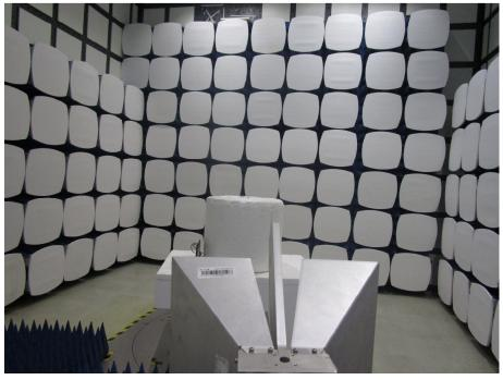
1.2 Radiated Spurious Emissions Test Setup
