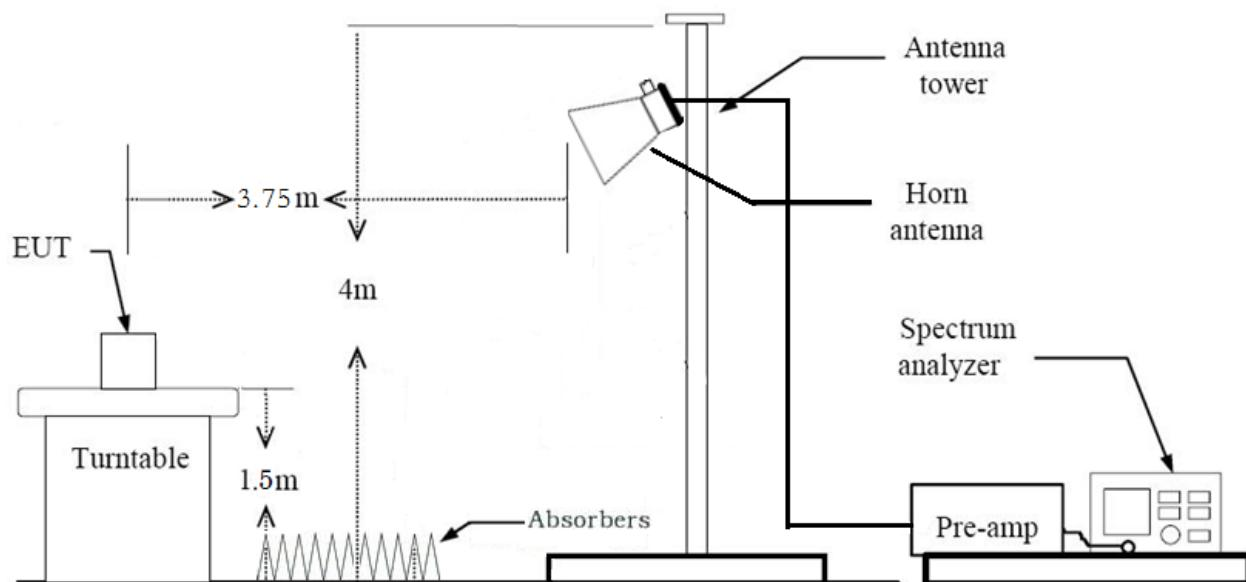
**Test Procedure of Radiated spurious emissions (Above 1 GHz)**
