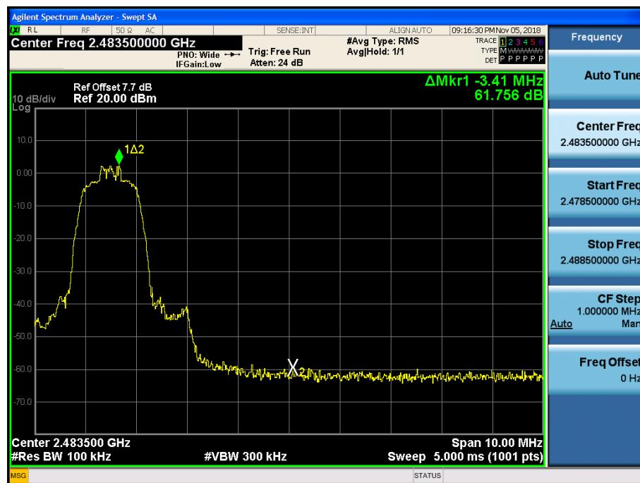
Test Plots with hopping (GFSK)
