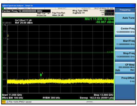
Test Plots (8DPSK)- 13 GHz – 15 GHz Spurious Emission (CH.78)
