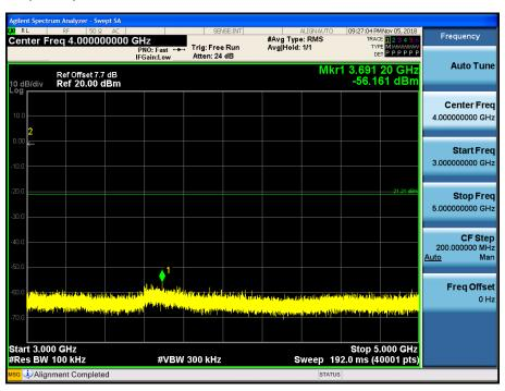
Test Plots (8DPSK)- 5 GHz - 7 GHz Spurious Emission (CH.78)
