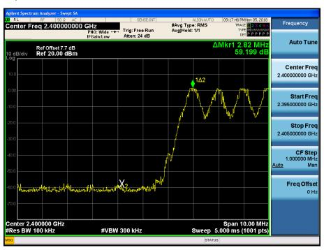
Test Plots with hopping (GFSK) Band Edges (CH.78)
