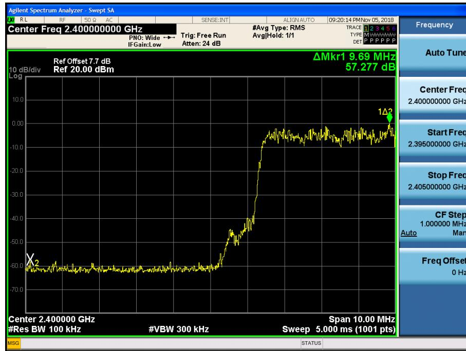
Test Plots with hopping (8DPSK)
