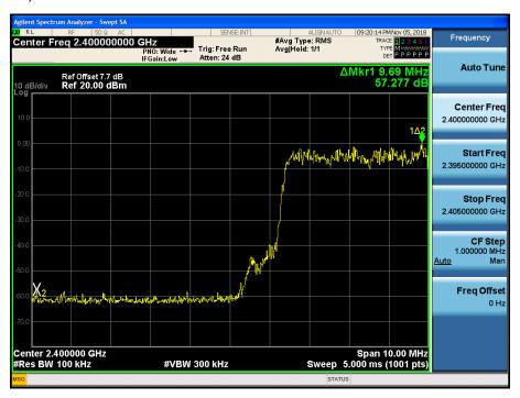
Test Plots with hopping (8DPSK) Band Edges (CH.78)
