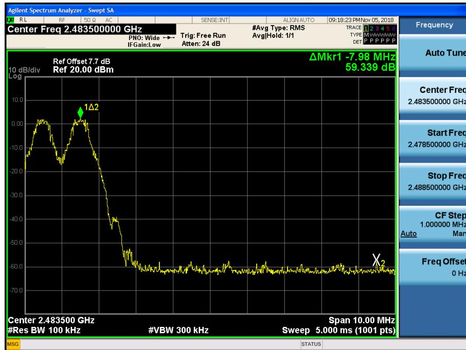
Test Plots with hopping (8DPSK)
