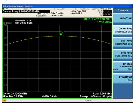
Test Plots (π/4DQPSK) Peak Power (CH.39)
