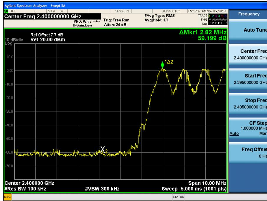
Test Plots with hopping (GFSK)
